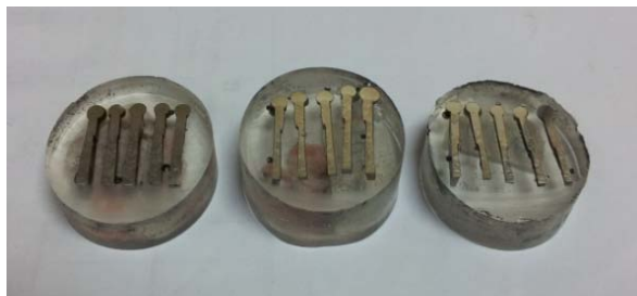
Fig. 7 : Photographs of prepared specimen for metallographic examination
