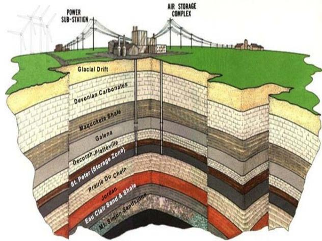
Figure 2 : Underground CAES backup by Wind Turbine Farm
