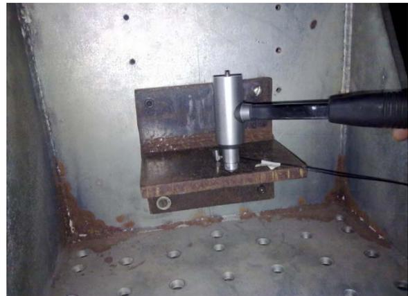
Fig. 3 : Experimental setup for Impact Hammer test
