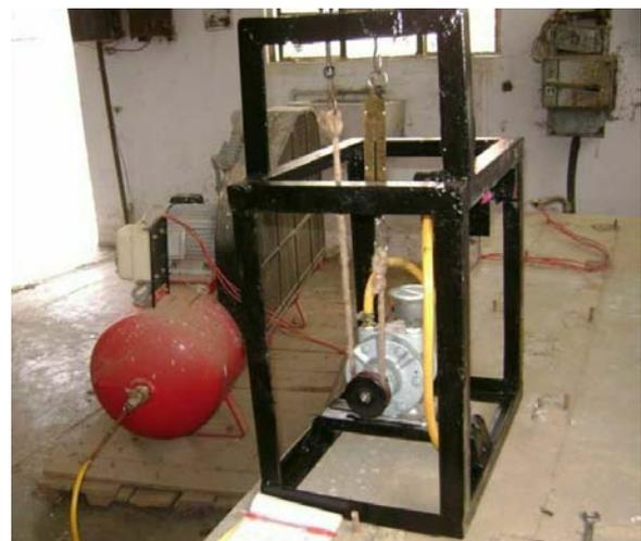
Fig. 10 : Actual test rig of air turbine
