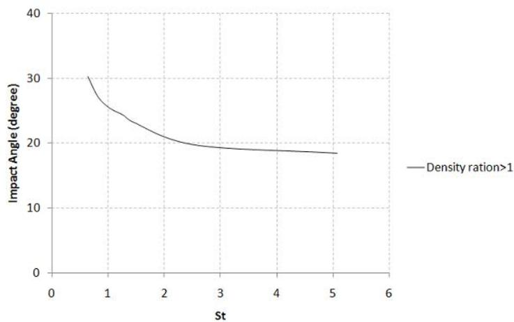
Fig. 10 : The angle between the particle impact direction and the tangent to surface at the bend wall during the particle impact for different Stokes number considering the density ratio is bigger than one
