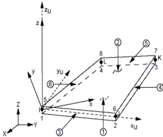
Fig.5 : SHELL63 Element Geometry
