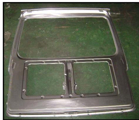
*Fig.2 :* A completed panel after press work
