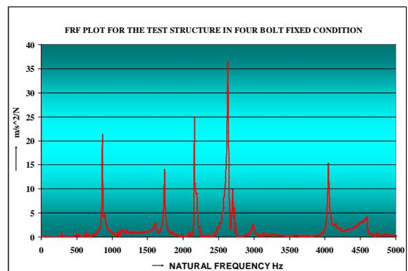
Fig.4 : Impact Hammer FRFs Measured from the Test Structure
