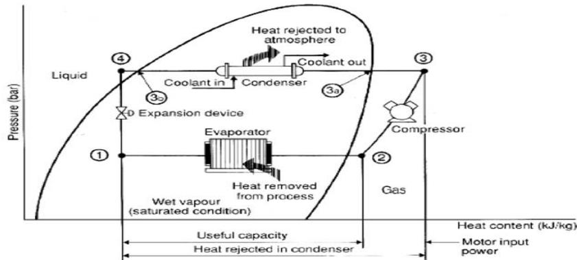
Fig. 1 : Schematic diagram of a Basic Vapour Compression Refrigeration System
