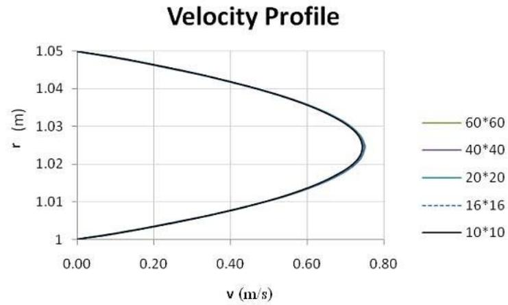
Fig. 2 : Velocity profile for grid independency study using different meshes
