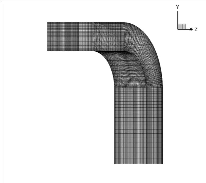
Fig. 3 : The bend curvature mesh configuration
