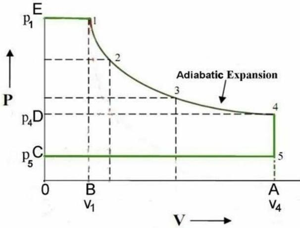
Figure 4 : Thermodynamic Processes (Isobaric, adiabatic and Isochoric Expansion)
