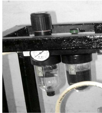
Fig. 9 : Air filter, regulator and lubricator
