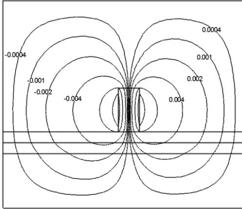
Fig. 2 : Magnetic field due to one rectangular magnet.
