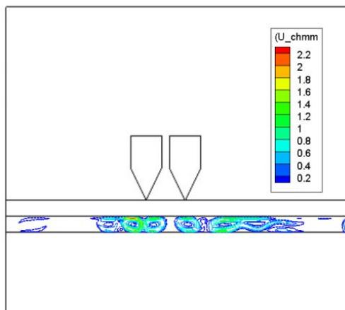
Fig. 10 : velocity field for two wedge shape magnet.
