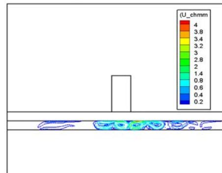
Fig. 6 : velocity field for one rectangular magnet
