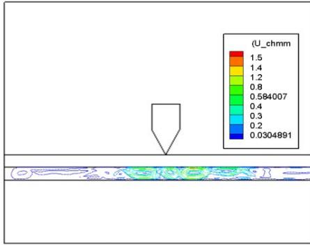
Fig. 8 : velocity field for one wedge shape magnet.
