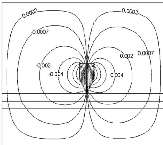
Fig. 4 : Magnetic field due wedge shape magnet.
