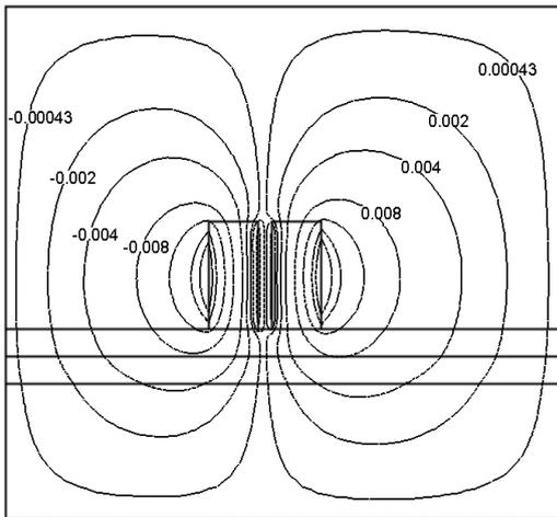
Fig. 3 : Magnetic field due to array of two rectangular magnets.
