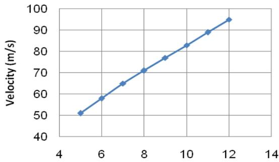
Figure 7 : effect of injection pressure on fuel velocity
