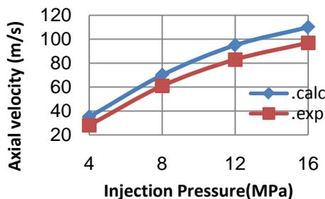
Figure 15 : comparison between experimental and theoretical axial velocity
