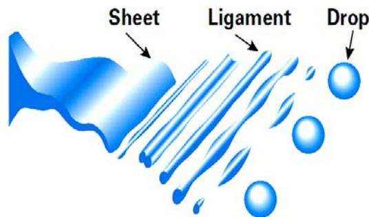
Figure 1 : Sheet disintegration and drop formation process[1]
