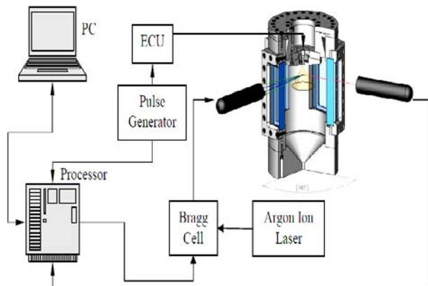
Figure 5 : Schematic of main components for PDA system
