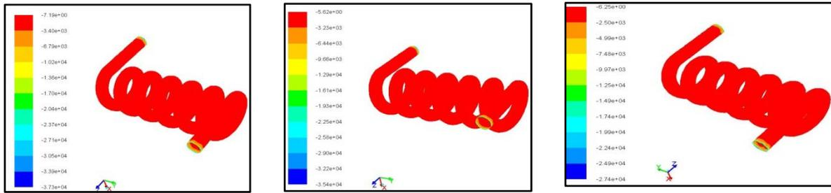
b) CFD-Results of Case-II( $Al_2O_3$  as a Nano fluid)
