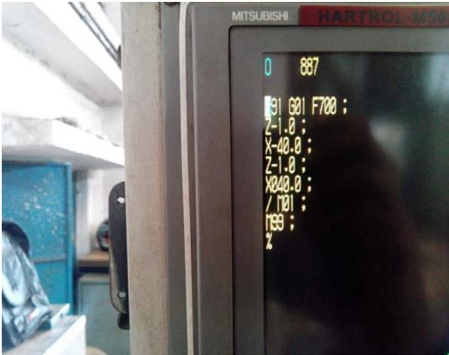
Figure 25 : G-code for Milling
