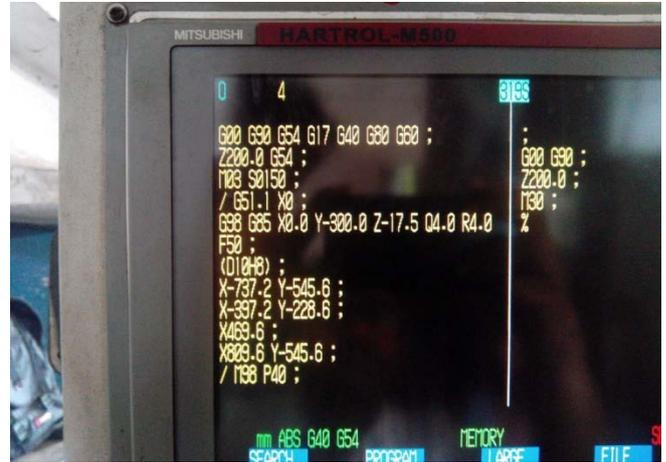
Figure 23 : G-code for Drilling
