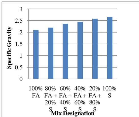
Fig. 2 : Specific gravity of fly ash and Sand mixtures
