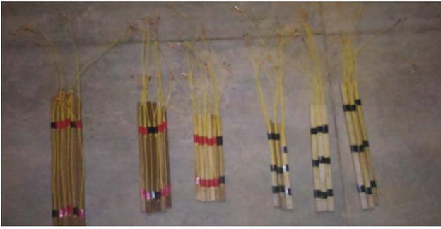
Figure 2 : Fixing of Thermocouple on wooden beads
