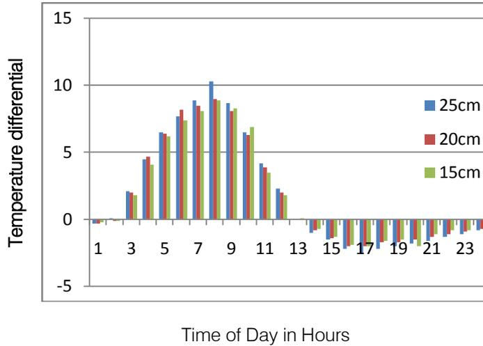
Figure 13 : Actual Temperature Differential at corner of HVFAC Slabs
