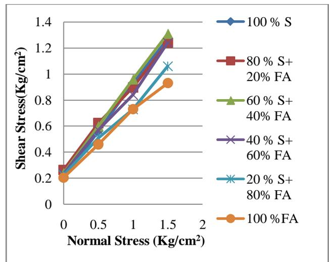
Fig. 5 : Direct shear test of Fly Ash and Sand Mixtures in Dry Condition
