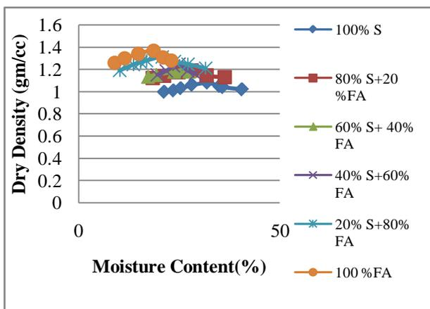
Fig. 3 : Compaction Curve of Fly Ash and Sand Mixtures
