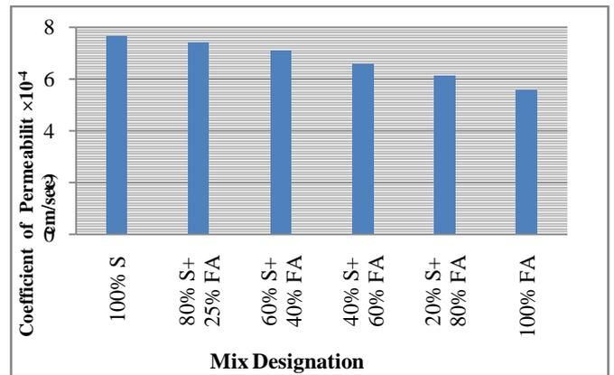
Fig. 4 : Coefficient of permeability of Fly Ash and Sand mixtures
