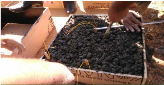
Figure 4 : Compaction of Concrete in Moulds
