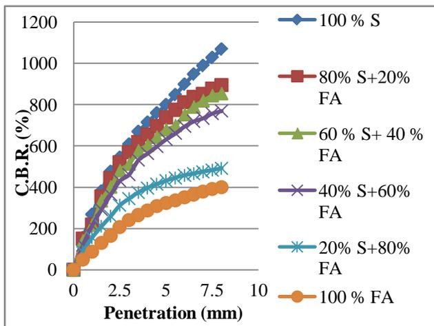
Fig. 7 : CBR value of Fly Ash and Sand Mixtures in Unsoaked Condition
