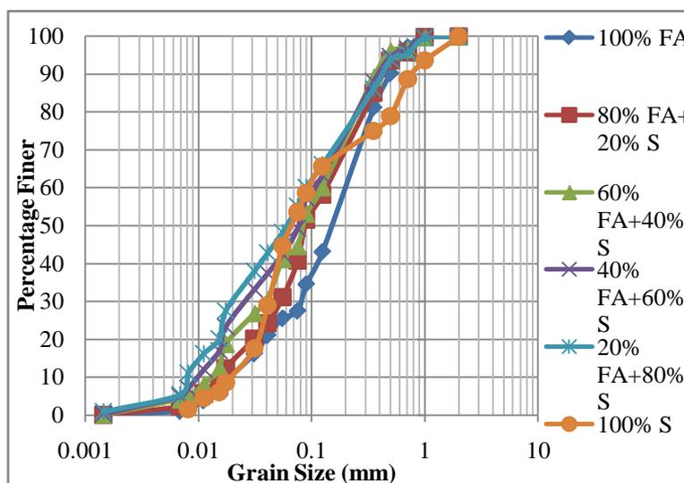
Fig. 1 : Grain Size distribution curve of Fly Ash and Sand mixtures
