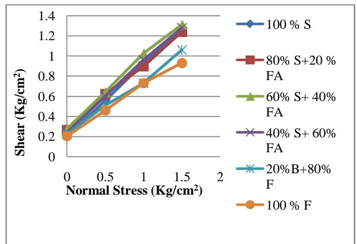
Fig. 6 : Direct shear test of Fly Ash and Sand Mixtures in Wet Condition
