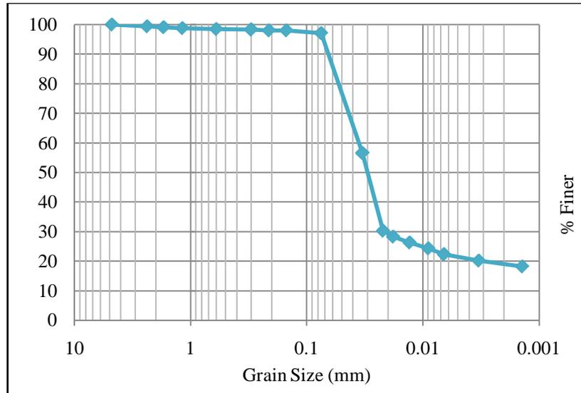
Figure 1 : Grain Size Distribution Curve of Soil
