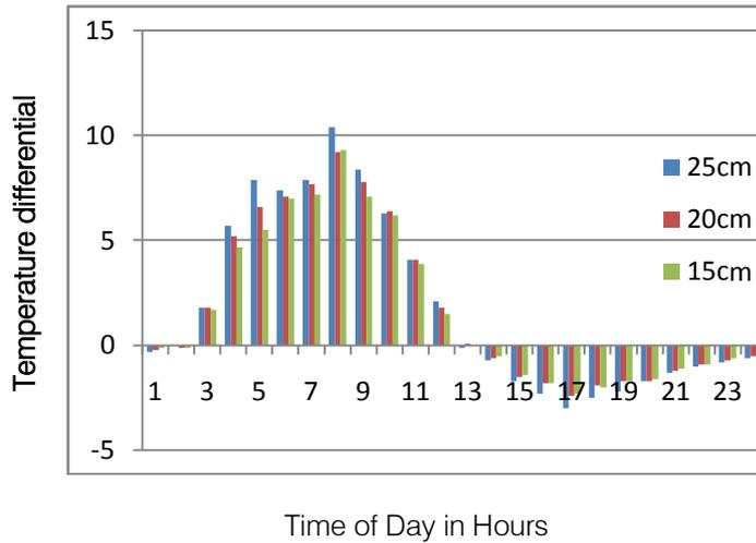
Figure 12 : Actual Temperature Differential at corner of PQC Slabs
