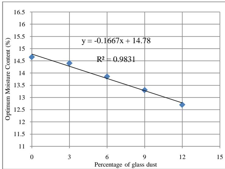
Figure 3 : Variation of Optimum Moisture Content with Percentage of Glass Dust
