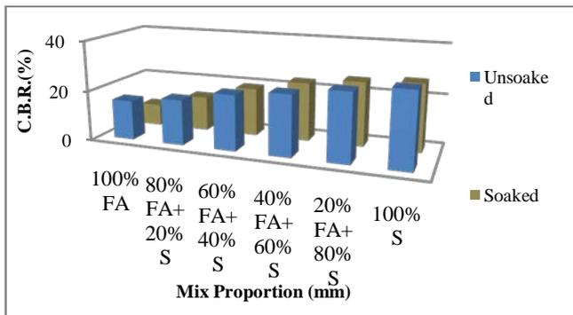
Fig. 9 : CBR value of mixtures of Fly Ash and Sand in soaked and Unsoaked Condition
