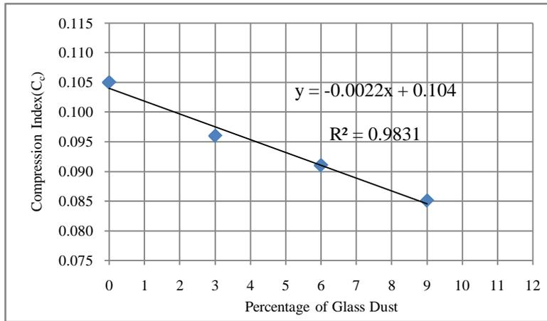
Figure 5 : Variation of Compression Index with Percentage of Glass Dust
