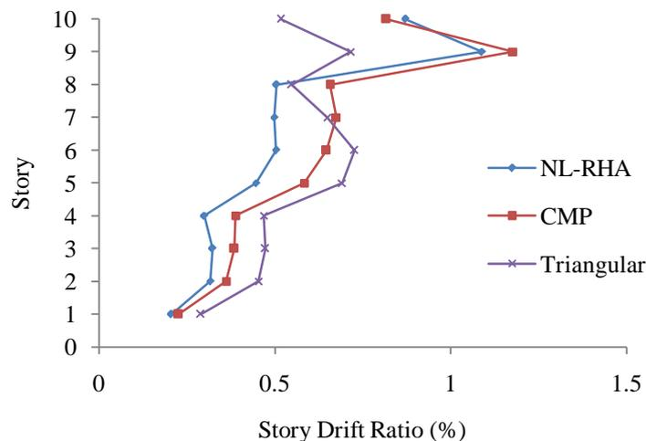
Figure 4.1 : Height-wise distribution of drift ratio for symmetric model
