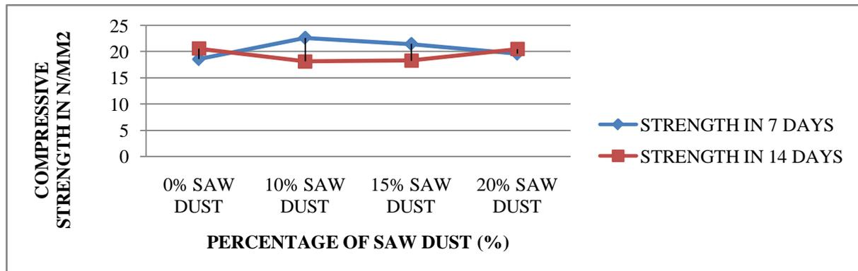
Figure 3 : Percentage of saw dust v/s Compressive strength
