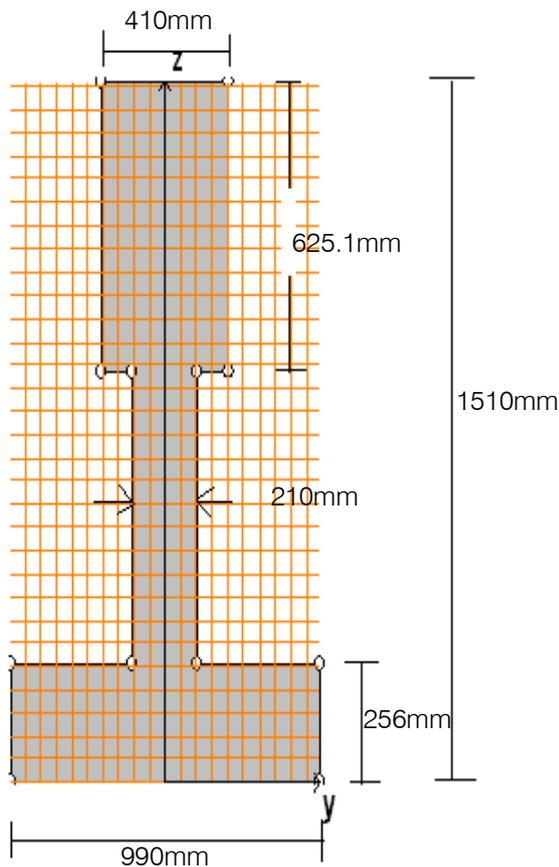
Figure 1 : Section of inverse-T girder
