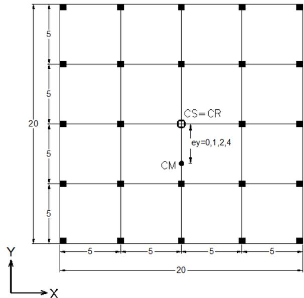
Figure 3.1 : Typical Plan of buildings considered (units in meters)
