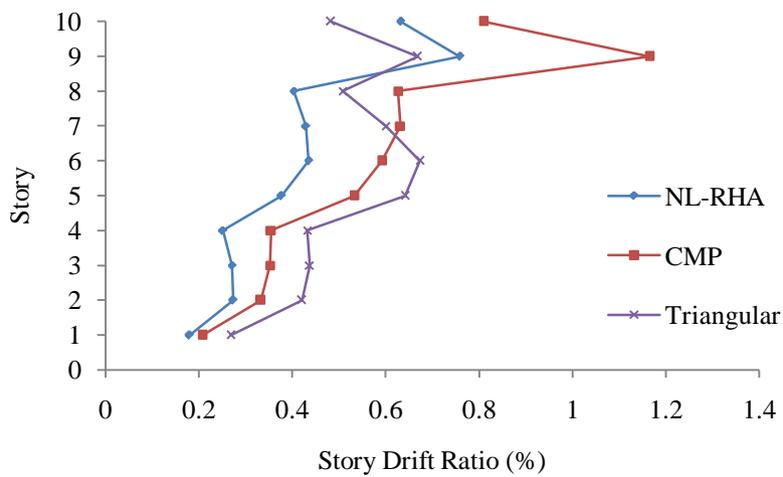
Figure 4.4 : Height-wise distribution of drift ratio for asymmetric model with 20% eccentricity
