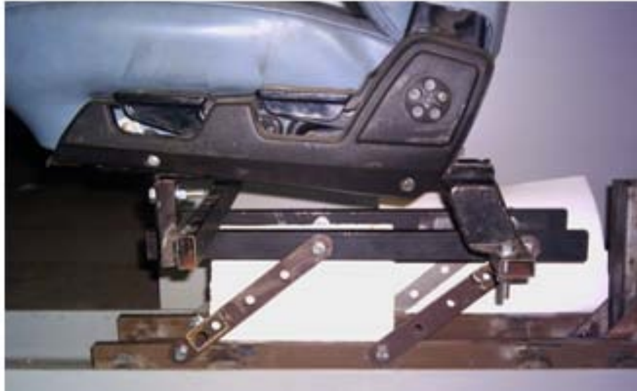
Figure 3 : Drop damping seat, (a) showing the linkages (b) the motion of the system during rear-end impact
