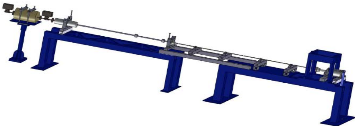
Fig.16 : Solid model of the entire SHPB setup
