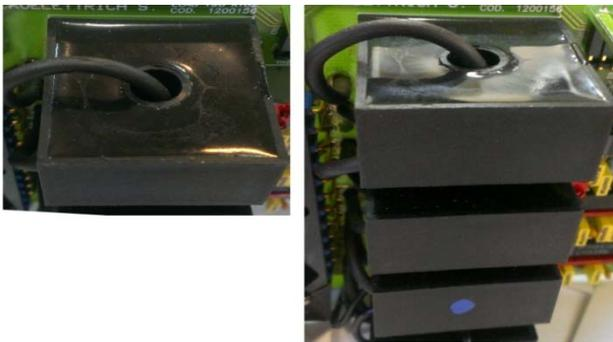
**Fig. 3 :** Encapsulated current transformers with epoxy encapsulated secondary winding hardened in vacuum. You can clearly see the primary winding, which consists of a single coil of flexible insulated wire
