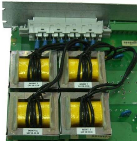
*Fig. 2 :* Example of a module of analogue inputs of DPR with installed CT. You can clearly see the primary winding, which consists of 4 coils of flexible insulated black wire
