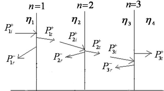
Figure 4 : Intrinsic Impedance Model
