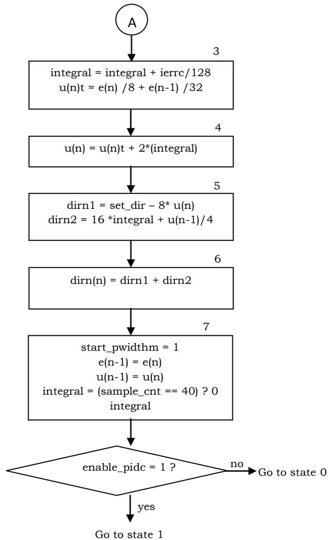
Figure 4 : ASM Chart for PID Controller Module
