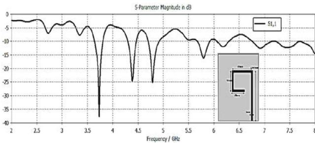
*Figure 3 :* Plot of reflection coefficient of Basic Monopole Rectangular Spiral Antenna (Simulated)
