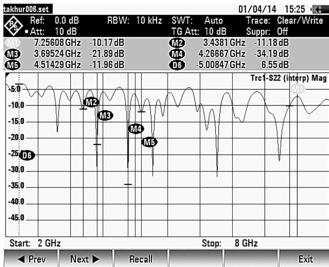
Figure 6 : Plot of reflection coefficient of increased turns Basic Monopole Rectangular Spiral Antenna (Tested on Rohde & Schwarz spectrum analyser)
