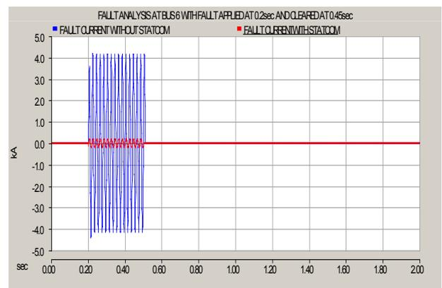
Figure 1.6b : Fault Current at Bus 6
