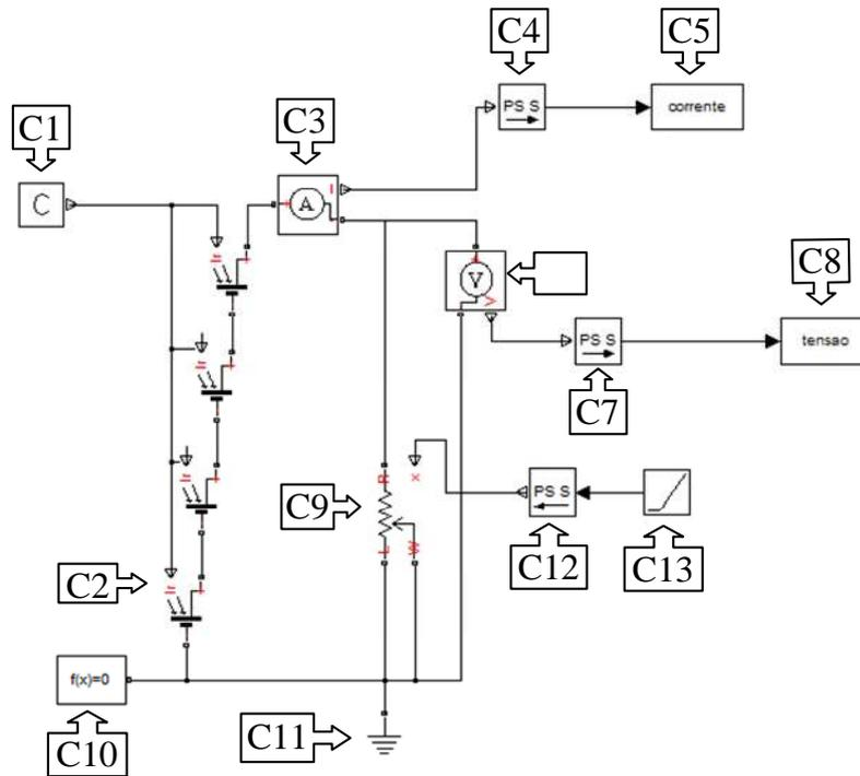
*Figure 2* : Model for a single face of the solar panel
