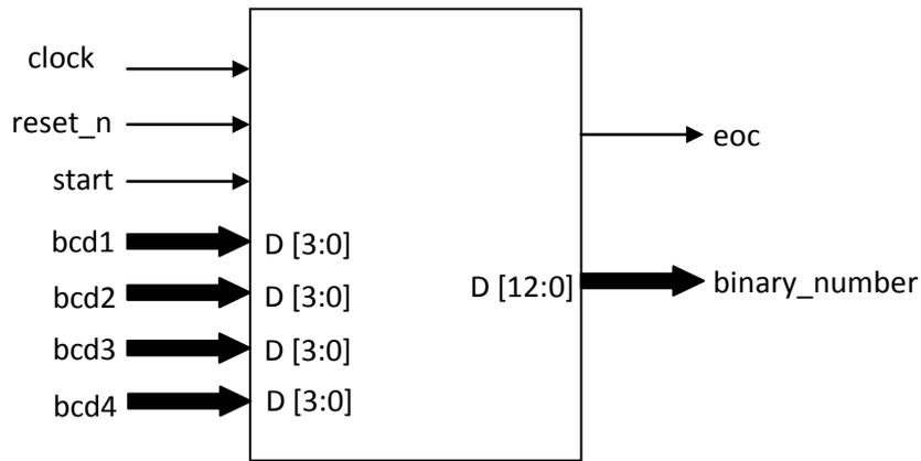
Figure 6 : BCD to Binary Converter Module
