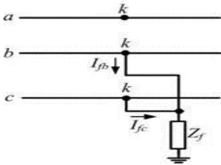
Figure 3 : Double line to Ground Fault
