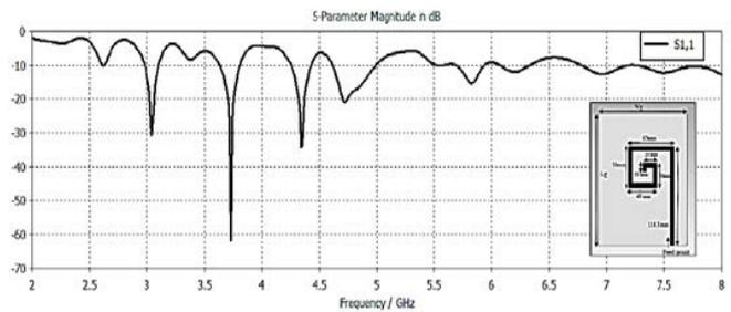
*Figure 4 :* Plot of reflection coefficient of increased turns Basic Monopole Rectangular Spiral Antenna (Simulated)
