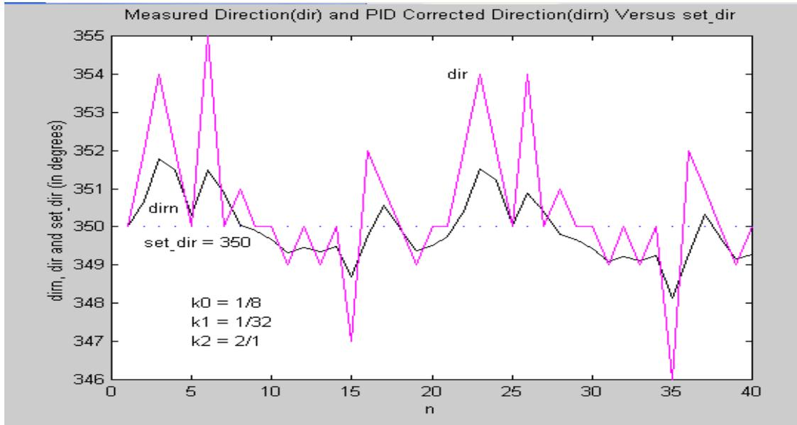
Figure 2 : Matlab Results: Comparison of PID Corrected Direction Vs Set Direction for Optimum Gain Constants – Least Error
