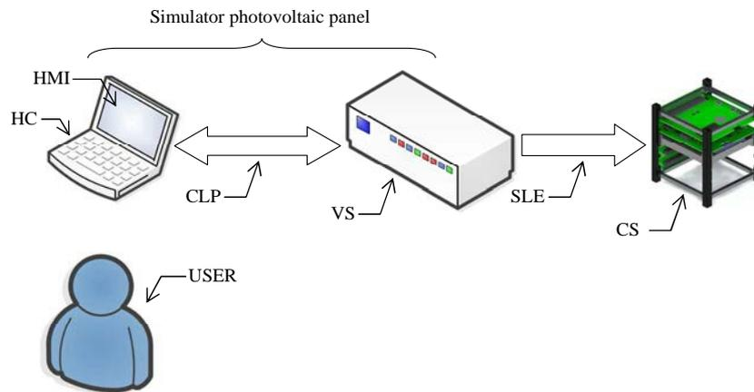
*Figure 1 : System components*
