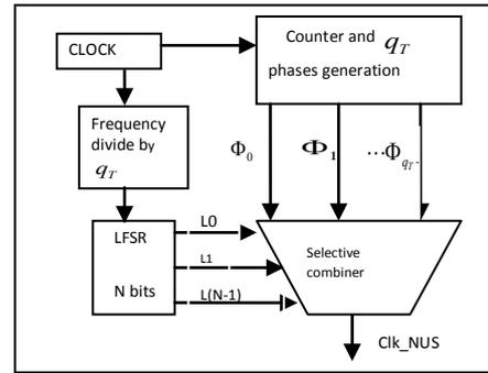
Figure 10 : Block Diagram for random clock
