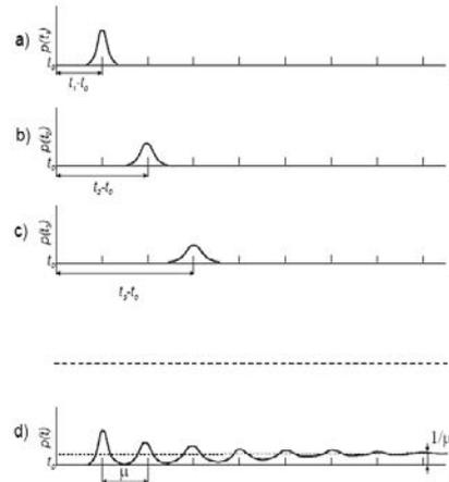
Figure 2: Probability density functions characterizing additive random sampling. a), b) c) probability density functions of a sum of 1, 2 and 3 time intervals, respectively; d) resulting sampling point density function
