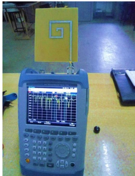
Figure 7 : Test setup for fabricated antenna
