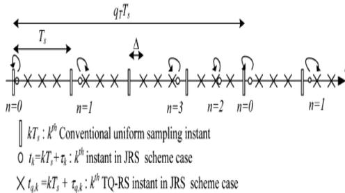
Figure 8 : Time-Quantized Random Sampling (TQ-RS) for  $q_T = 4$
