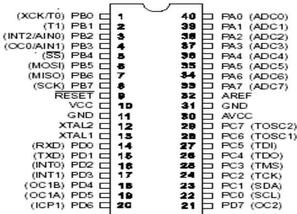
Figure 6 : Atmega16 microcontroller
