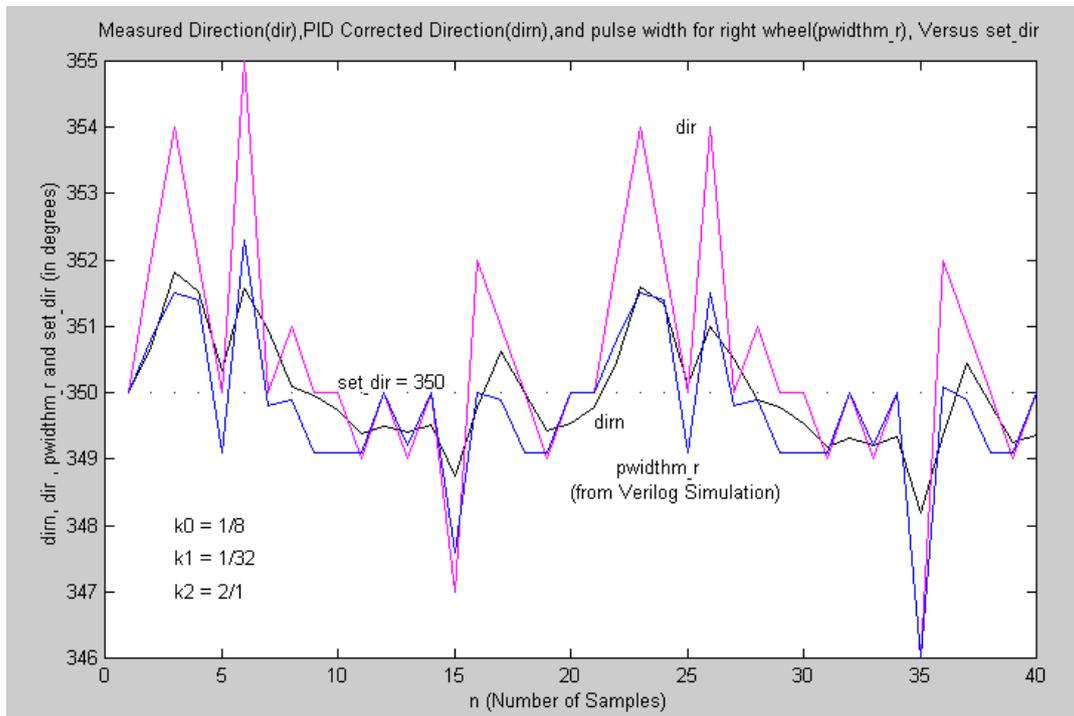
Figure 10 : Robot Controller Verilog RTL Design Validation Using Matlab
