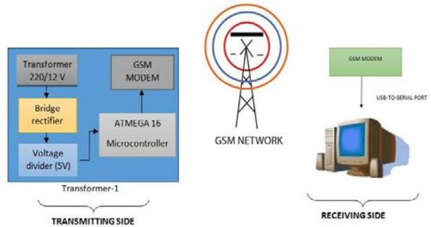
Figure 4 : Block diagram arrangement of the project
