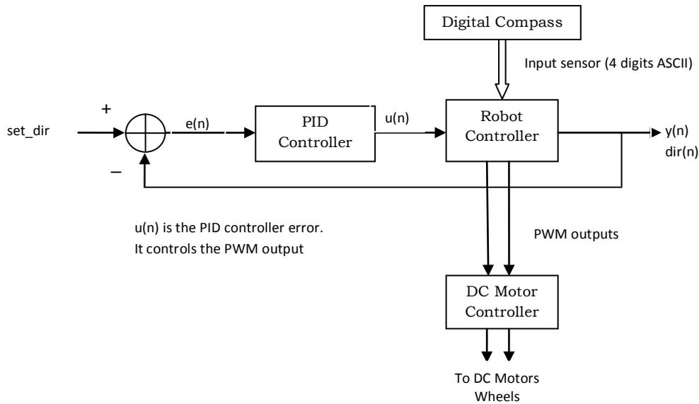
Figure 3 : Block Diagram of the Robotic Vehicle with PID Control
