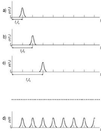
Figure 1: Probability density functions characterizing periodic sampling with jitter. a), b) c) probability density functions of a sum of 1, 2 and 3 time intervals, respectively; d) resulting sampling point density function
