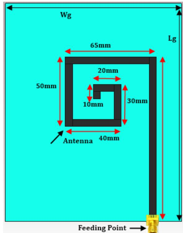
Figure 2 : Increased turns rectangular microstrip spiral antenna
