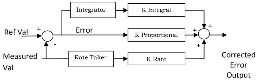
Figure 1 : Block Diagram of PID Controller
