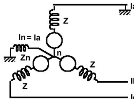
Figure 1 : Single Line to Ground fault
