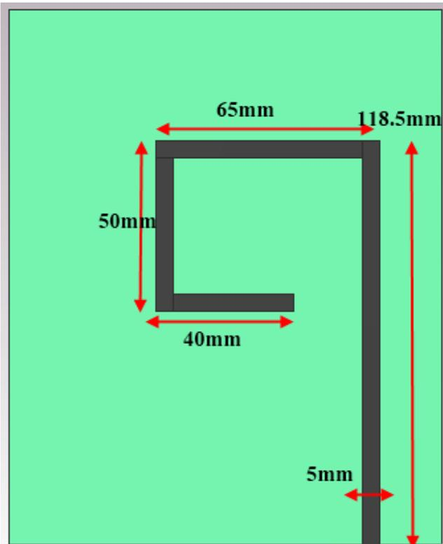
Figure 1 : Basic rectangular microstrip spiral antenna and its dimensions
