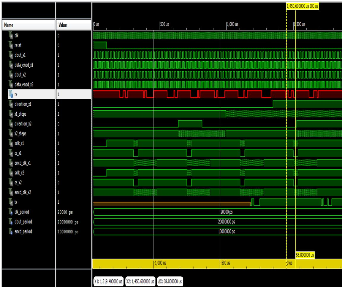
Figure 4 : Results for collimator control that states about the steps and direction control of stepper motor and also about the feedback from encoders
