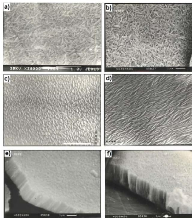
**Figure 2 :** Microfotographs of the surface of (a-d) and cleavages (e, f) coating MoS<sub>2</sub> (a, c, e) and WSe<sub>2</sub> (b, d, f), applied at a temperature of 523 K (MoS<sub>2</sub>) to 653 K (WSe<sub>2</sub>) at location samples in the center of the plate (a, b, e, f) and on its periphery (c, d)
