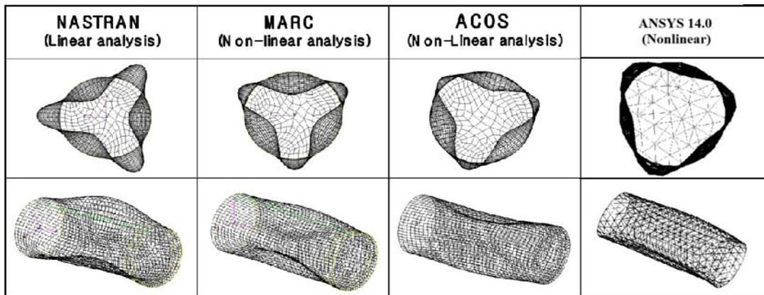
Figure 5 : Buckling modes of the  $[\pm 45/90]$  FW composite cylinder
