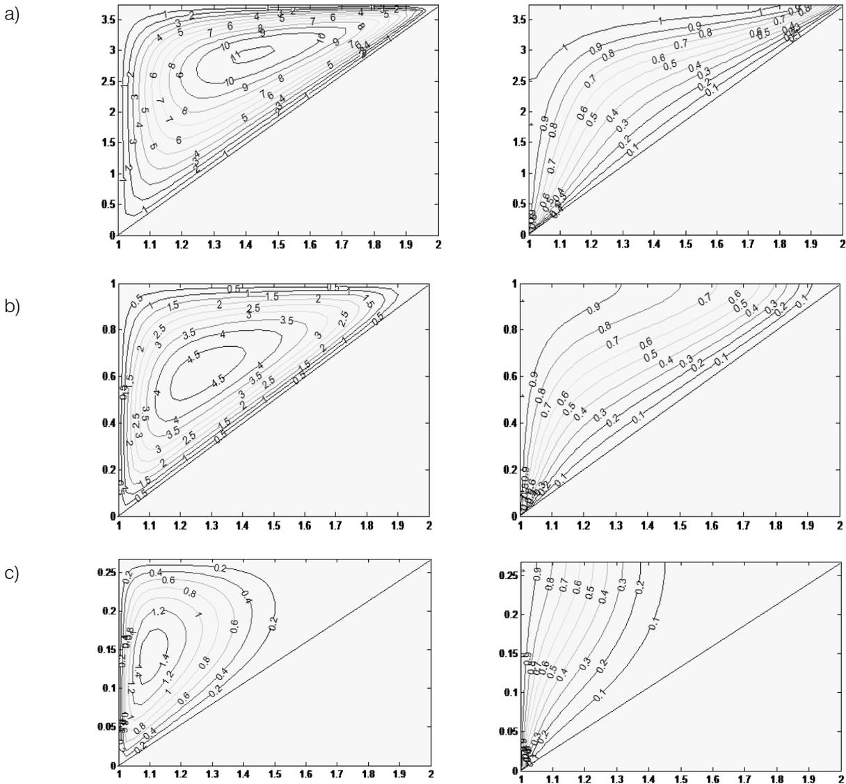
Figure 1 : Streamlines (left) and Isotherms (Right) for  $Ra=100, R_r=1, \epsilon=0.01$
