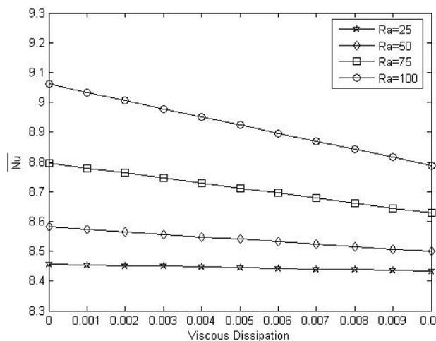
Figure 10 :  $\overline{Nu}$  variations with  $\epsilon$  at hot surface for different values of Ra at  $C_A = 75, R_r = 1$
