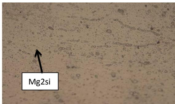
Figure 5 : microstructure at 450°C and 0.2s<sup>-1</sup>
