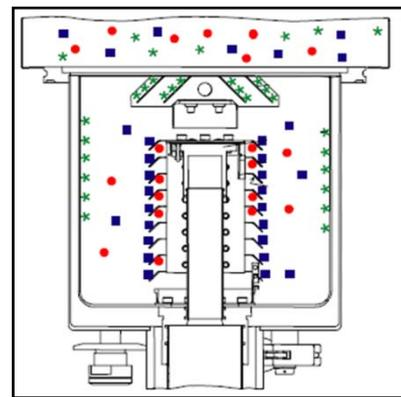
Figure 9 : Schematic of Cryo-genic Pump working principle
