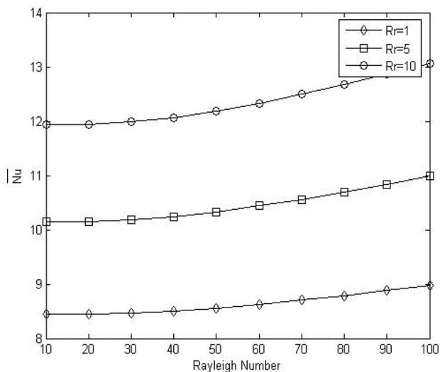
Figure 6 :  $\overline{Nu}$  variations with Ra at hot surface for different values of  $R_r$  at  $C_A=75, \epsilon=0.01$
