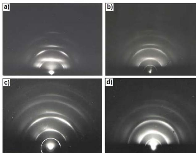
**Figure 1 :** The electron diffraction patterns of coatings MoS<sub>2</sub> (a, c) and WSe<sub>2</sub> (b, d) a thickness of 0.5 microns, applied at a temperature 523 K (MoS<sub>2</sub>) and 623 K (WSe<sub>2</sub>), and the location of samples in the center of the plate (a, b) and at its periphery (c, d)
