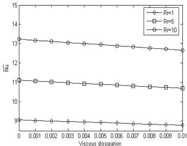
Figure 9 :  $\overline{Nu}$  variations with  $\epsilon$  at hot surface for different values of  $R_r$  at  $C_A = 75, Ra = 100$
