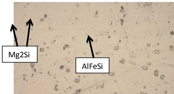
Figure 4 : microstructure at 350 and 0.2s<sup>-1</sup>
