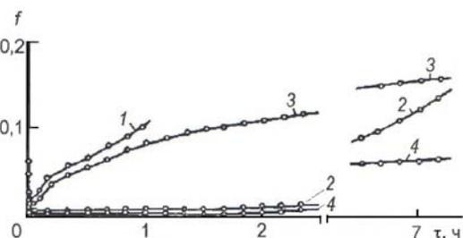
Figure 6: Dependence of the friction coefficient on the duration of the test coatings: 1 - MoS<sub>2</sub>; 2 - MoS<sub>2</sub>D<sub>x</sub>; 3 - (Mo<sub>2</sub>N- M<sub>k</sub>N<sub>m</sub>X<sub>n</sub> - MoS<sub>2</sub>); 4 - (Mo<sub>2</sub>N- M<sub>k</sub>N<sub>m</sub>X<sub>n</sub> - MoS<sub>2</sub>D<sub>x</sub>)
