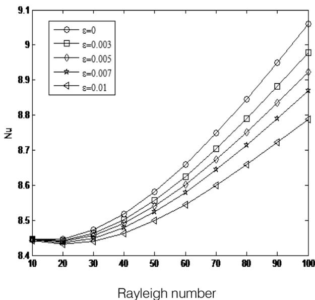
Figure 7 :  $\overline{Nu}$  variations with Ra at hot surface for different values of  $\epsilon$  at  $C_A = 75, R_r = 1$
