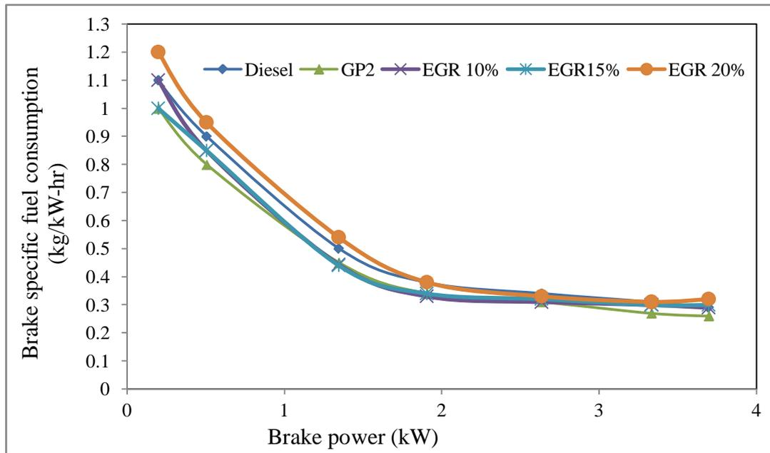
Figure 2 : Comparison of Brake specific fuel consumption with different percentages of EGR
