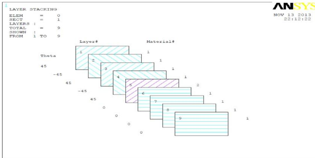
Figure 2 : Layer stacking sequence of composite pressure vessel  $[\pm 45/0]$  FW
