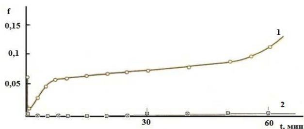
Figure 5: Coefficient of friction on the duration of the test coatings doped MoS<sub>2</sub> (1 - MoS<sub>2</sub>; 2 - MoS<sub>2</sub>D<sub>x</sub>)
