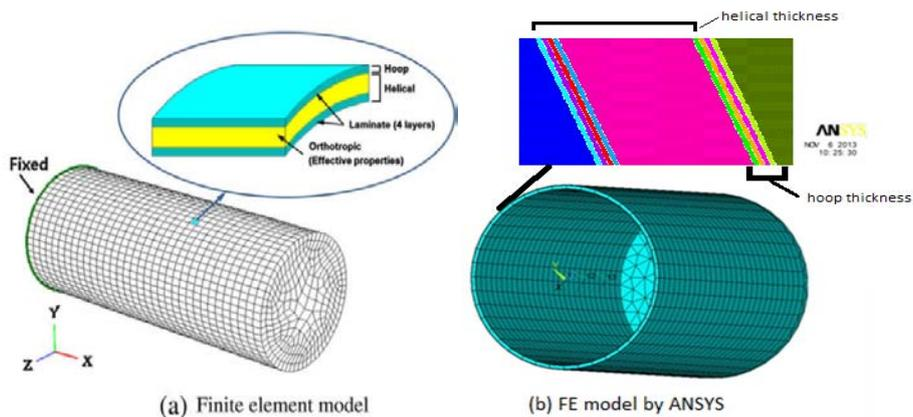
Figure 3 : (a) Finite element model by ACOS win. (b) Finite element model by ANSYS APDL
