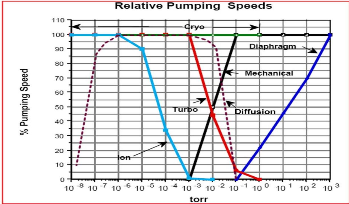
Figure 10 : The change of relative pumping speed with pressure of some common vacuum pumps [7]
