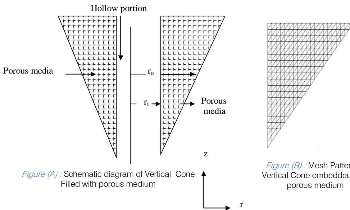
Figure (A) : Schematic diagram of Vertical Cone Filled with porous medium
