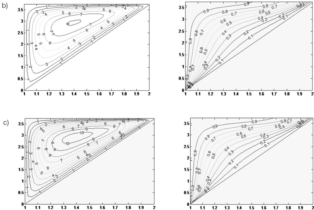
Figure 4 : Streamlines (left) and Isotherms (Right) for  $\epsilon=0.003, C_A = 15, R_r=1$
