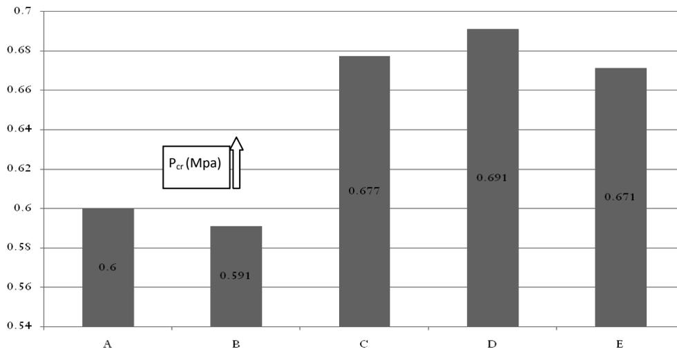
Figure 7 : Bar graph (a) experimental test result (b) result obtained by Ansys (c) result obtained by Nastran (d) result obtained by Marc (e) result obtained by ACOSwin
