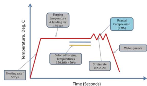
**Figure 1 :** Gleeble cycle for 6061 Aluminium Alloy
