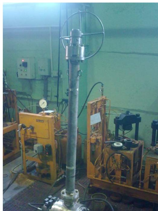
Figure 4 : Drive of the ball valve DU-160 with extension column
