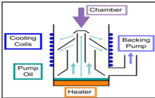
Figure 6 : Schematic of Diffusion Pump working principle
