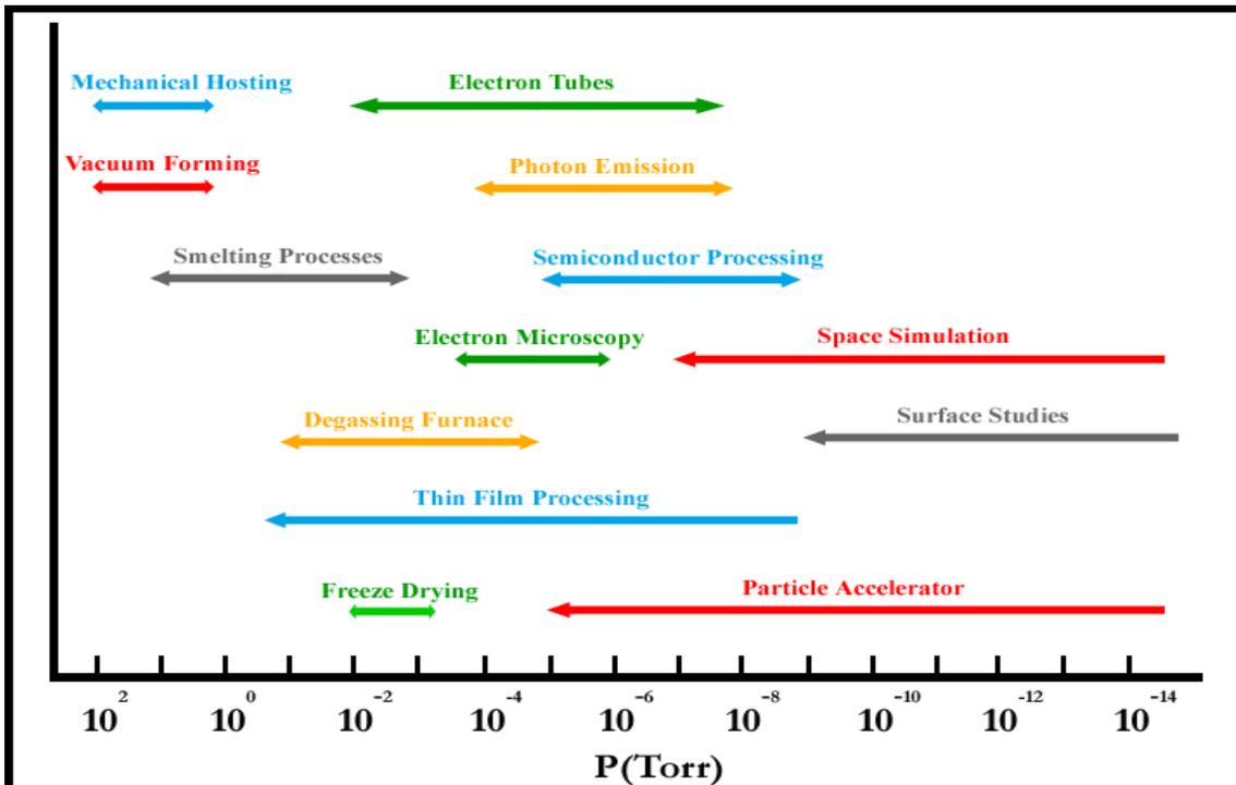
Figure 1 : Vacuum applications in different vacuum ranges [1]
