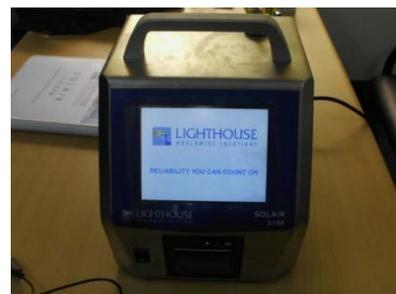
Figure 2 : Solair-3100 1.0 Cfm Optical Particle Counter
