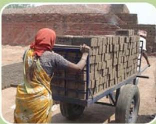
The bricks are carried to the kiln for heating process in a trolley (hand pulled). It carries 250 bricks at once.
