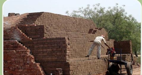
Brick pyramid is covered on the sides by faulty bricks or damaged bricks and sides are stuffed with coal.
