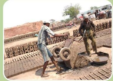
A worker is assigned the job of moulding clay into bricks
