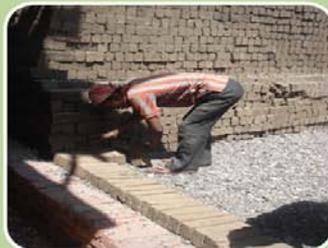
A layer of coal pieces is spread after two layers of bricks.
