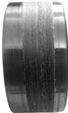
Figure 2: The anti-friction layer formed on the surface of the counterbody in the process of friction of the sample №4 of the hybrid composite
