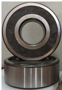
Figure 3: Rolling bearing № 62306 with AFF, sample № 4
