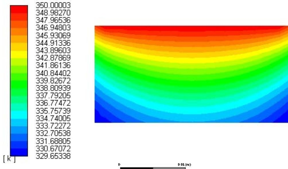
Figure 2: Static Temperature Contour for Water with heat transfer coefficient of 3000 W/m<sup>2</sup>-K
