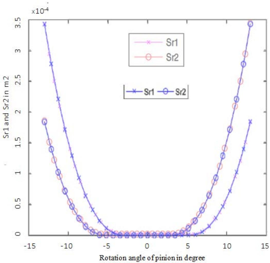
Figure 13: Superposition of radial leakage surfaces from our model (in blue) and those from Abdelilah Lasri's model [13] (in red color)
