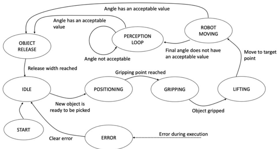
Fig. 7: State Machine with transition conditions
