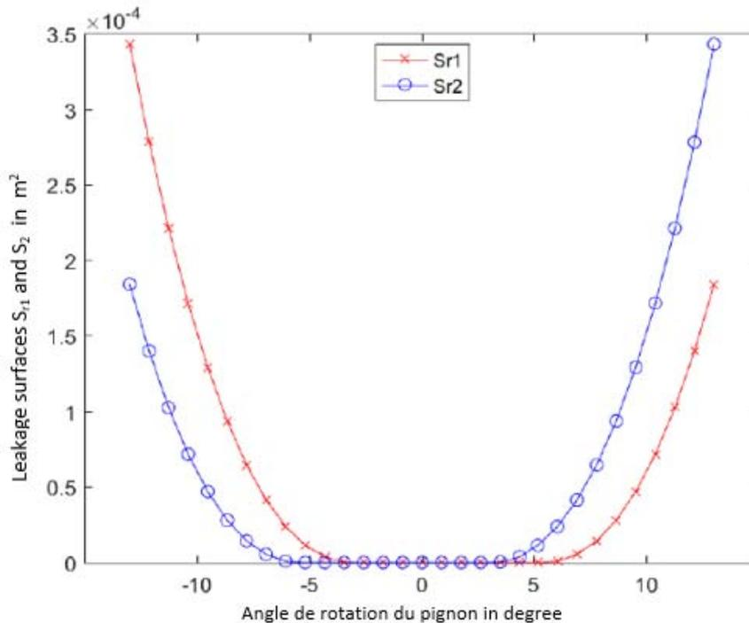
Figure 11: Evolution of the radial leakage surfaces 1 and 2 as a function of the angle of rotation of the driver gear. Case of the gearing system of table 2
