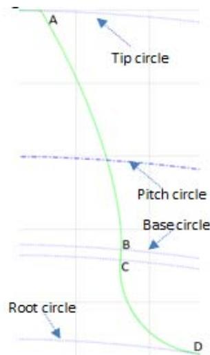
Figure 8: Detailed view of the half of tooth profile of gear 1 of table 1. Here  $r = 93,9693\text{mm}$ ;  $r_f = 89,5\text{mm}$
