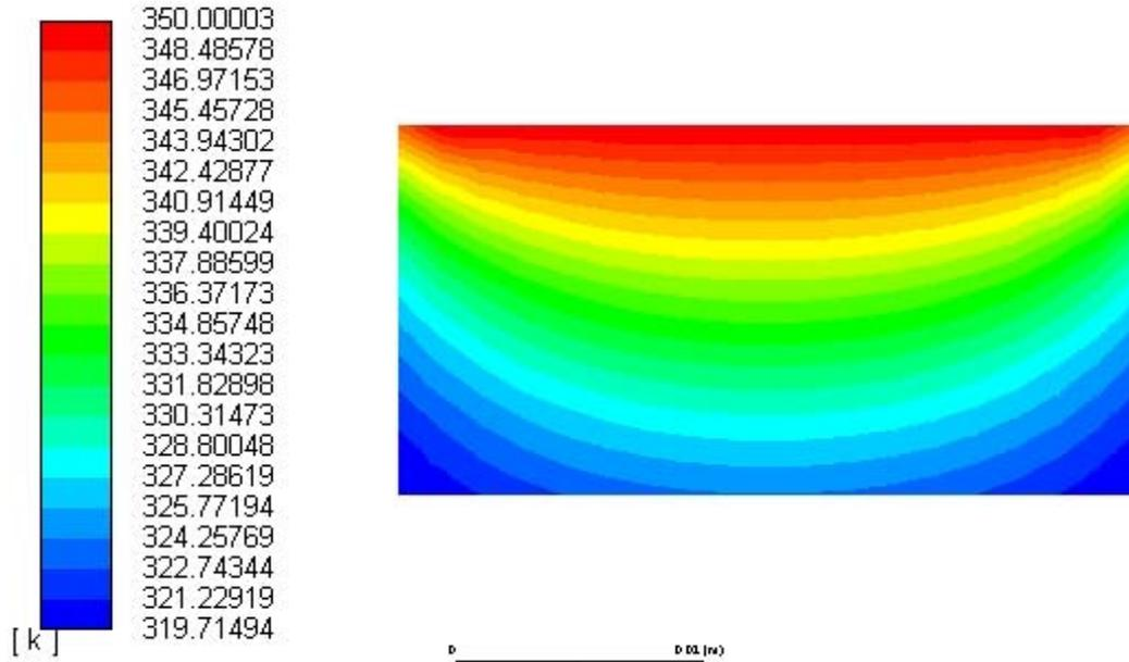
Figure 3: Static Temperature for Al-Ox Nanofluid with heat transfer coefficient of 9000 W/m<sup>2</sup>-K
