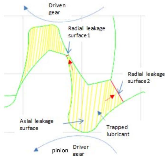
Figure 1: Inter-tooth space and trapped lubricant
