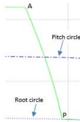
Figure 10: Detailed view of the half of the tooth in gear 3 of table 1. Here  $r = 142.8333\text{ mm}$ ;  $r_f = 147\text{ mm}$
