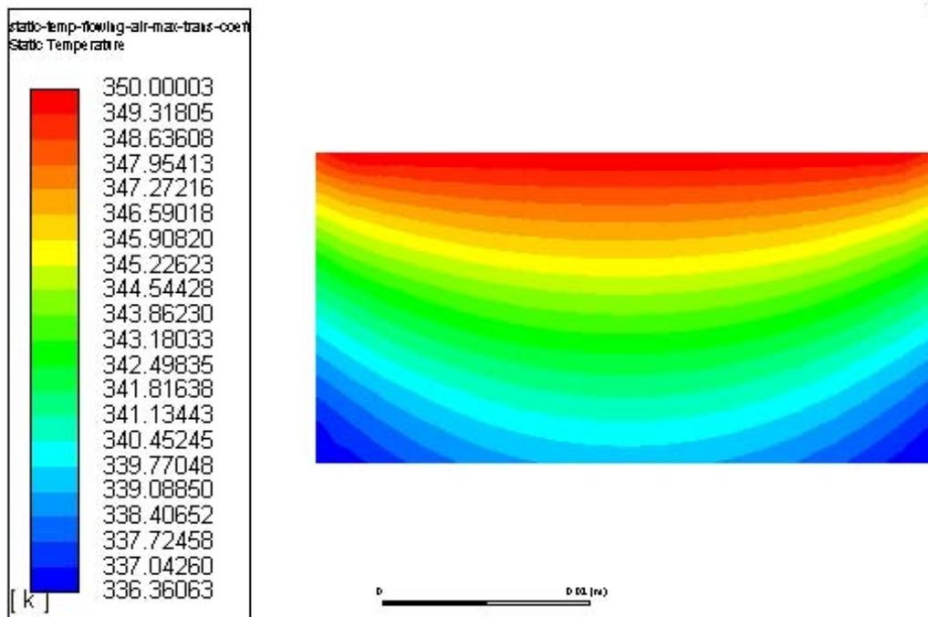
Figure 1: Static Temperature Contour for air with heat transfer coefficient of 1000 W/m<sup>2</sup>-K
