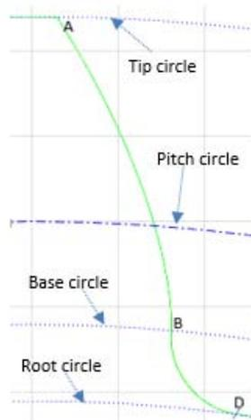
Figure 9: Detailed view of the half of the tooth of gear 2 in table 1. Here,  $r = 187.9385\text{ mm}$ ;  $r_f = 185.5\text{ mm}$
