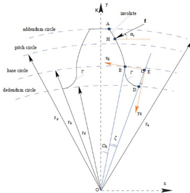
Figure 4: Geometry of an external spur gear
