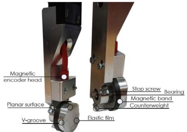
Fig. 2: Detail of the jaw provided of balancing mass and magnetic encoder
