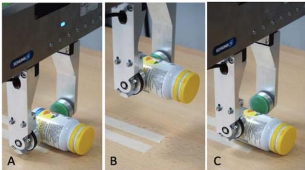
Fig. 3: Main sequence for moving a cylindrical object without alignment: (A) gripping with v-shaped cavity parallel to the ground, (B) lifting with fixed object, (C) releasing without movement of the jaw disks
