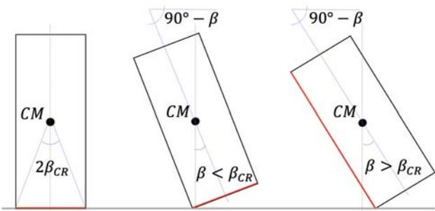
Fig. 9: Geometric condition for alignment success (cone of stability) with  $\beta$  the package's angle with the vertical plane and  $\beta_{cr}$  the threshold angle for stability. In red the final stability side of the package after release
