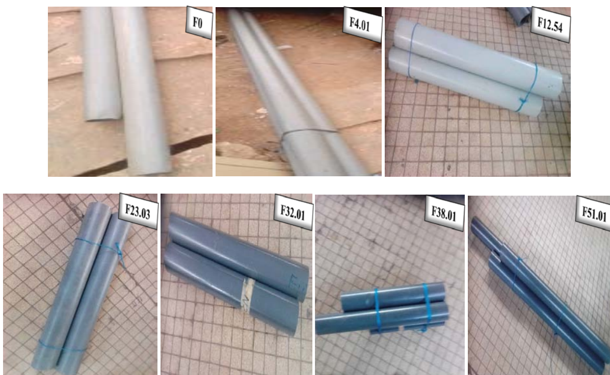
Figure 1: Unloaded PVC tubes and PVC tubes loaded with micronized dura palm kernel shell powder.
