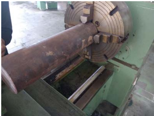
Fig. 1: (a). EN36C Steel mounted on the lathe.
