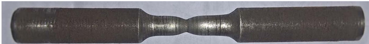
Fig. 2(b): ASTM-E8 EN36C steel Specimen (Broken) after the tensile test.
