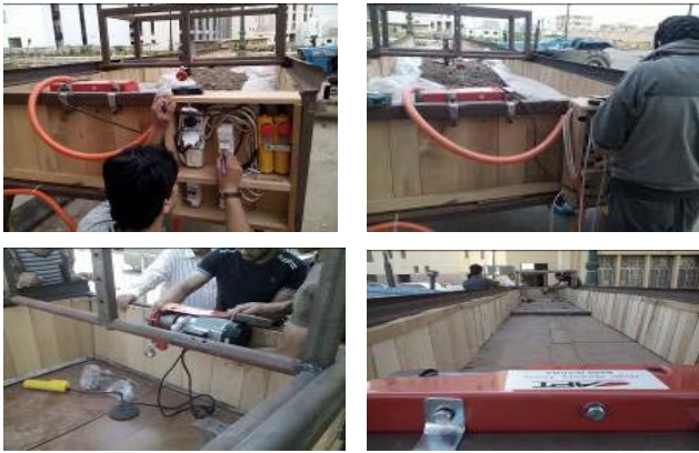
Figure 2: Installing soil bin and attached control units and motors
