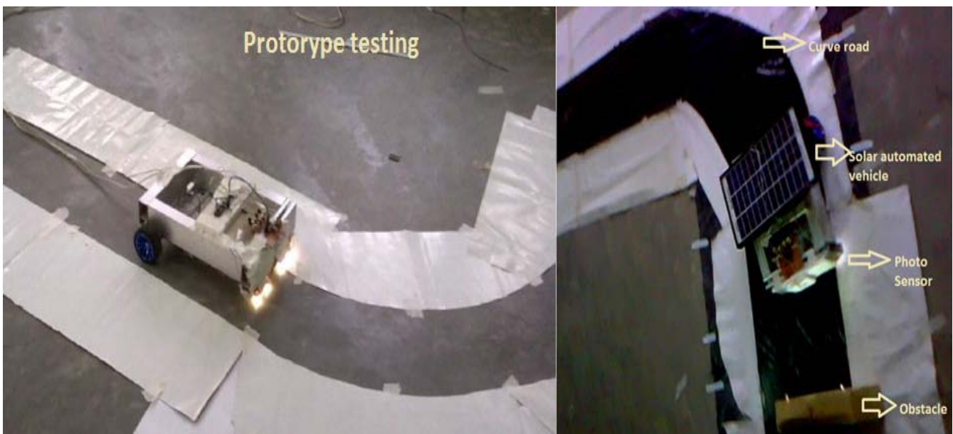
Figure 12 : Prototype vehicle testing (on the left) & three photosensor based automated solar vehicle on the road
