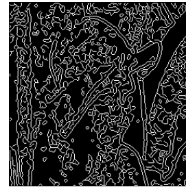
Fig 5.4 : Detection of edges using Fuzzy-Canny edge detector
