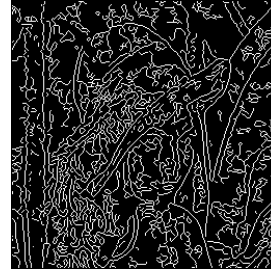
Fig 5.2 : Detection of edges using Canny edge detection
