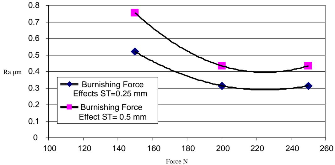
Figure 4 : (b) The effect of burnishing force on the surface roughness under high table speed (=120 mm/min)
