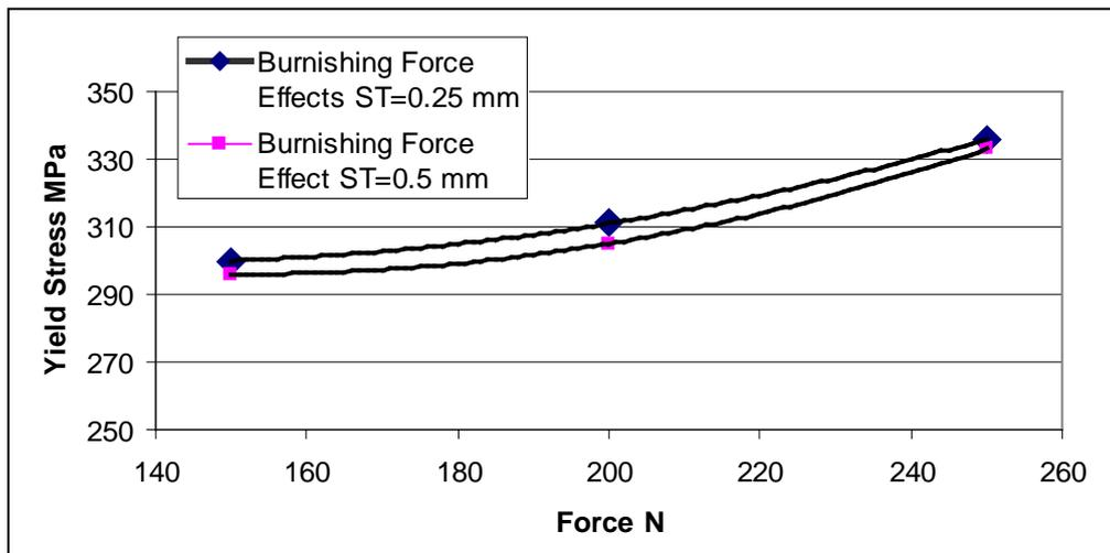
Figure 7: (b) The effect of burnishing force on the bending stress at high table speed
