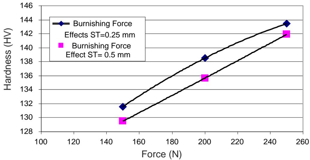
Figure 5 : (a) The effect of burnishing force on the Surface Hardness under low table speed
