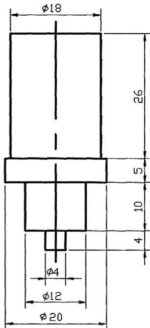
Figure 1 : Welding tool dimensions
