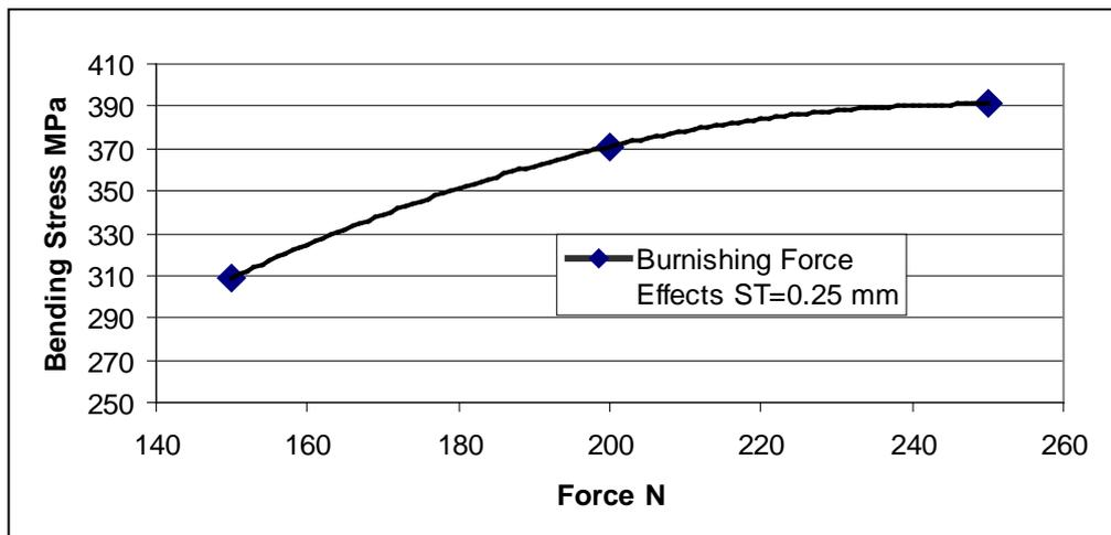
Figure 6 : The effect of burnishing force on the bending stress
