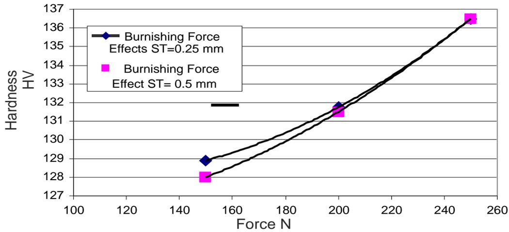
Figure 5 : (b) The effect of burnishing force on the Surface Hardness under high table speed
