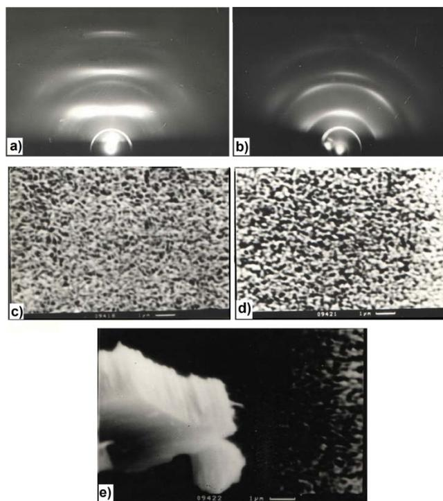
Figure 7: Electron diffraction (a, b) and micrographs (x5000) (c, d, e) coating WS<sub>2</sub>Ga<sub>x</sub>
