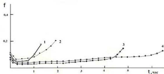
Figure 8: Dependence of the friction coefficient on the duration of the test doped coatings WS<sub>2</sub> and WSe<sub>2</sub> with wear sublayer Cr<sub>2</sub>O<sub>3</sub>, deposited on titanium alloys: (1 - WS<sub>2</sub>; 2 - WSe<sub>2</sub>; 3 - WSe<sub>2</sub>Ga<sub>x</sub>; 4 - WS<sub>2</sub>Ga<sub>x</sub>)
