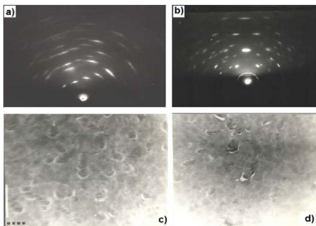
**Figure 4 :** Electron diffraction (a, b) and micrographs (x5000) (c, d) coating AlN (a, c) and Cr<sub>2</sub>O<sub>3</sub> (b, c, d)
