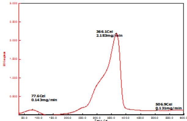
Figure 5 : DTG curve for Acrylonitrile of 2 Mconcentrated treated neem wood
