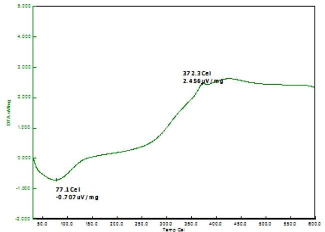
Figure 17 : DTA curve for Acrylonitrile of 2M concentrated treated cork wood
