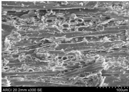
Figure 31 : Microscopic view poly acrylonitrile affinity of 2M concentration treated neem wood
