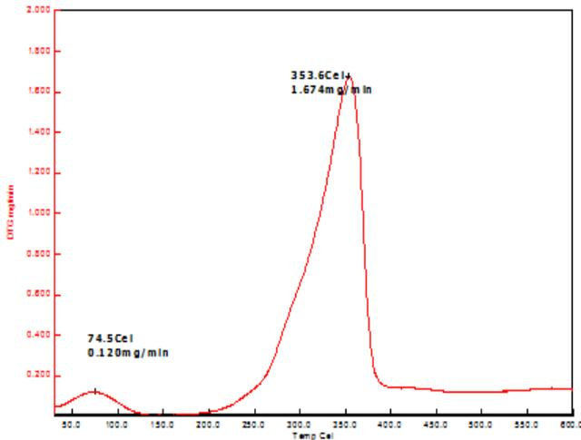
Figure 18 : DTG curve for Acrylonitrile of 2M concentrated treated cork wood
