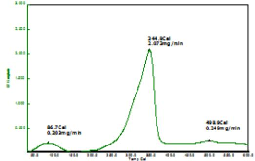
Figure 8 : DTG curve for Acrylonitrile of 4 Mconcentrated treated neem wood
