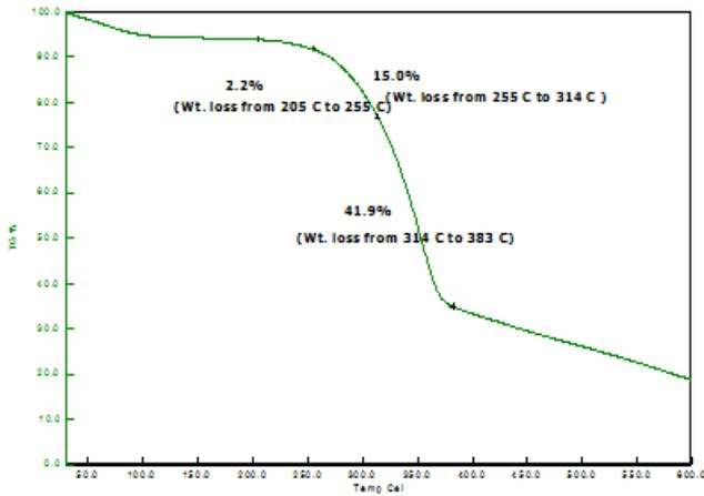
Figure 19 : TGA curve for Acrylonitrile of 2M concentrated treated cork wood
