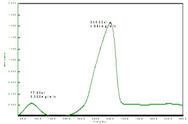
Figure 21 : DTG curve for Acrylonitrile of 4M concentrated treated cork wood
