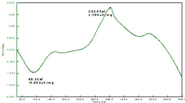
Figure 3 : D TA for Untreated neem wood
