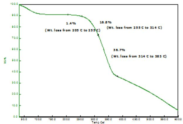
Figure 16 : TGA for Untreated cork wood
