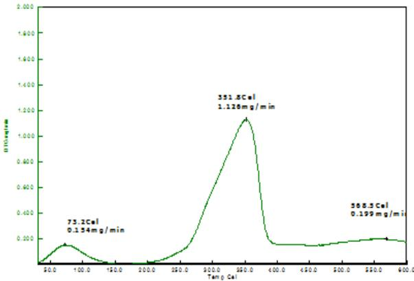
Figure 24 : DTG curve for Acrylonitrile of 6M concentrated treated cork wood
