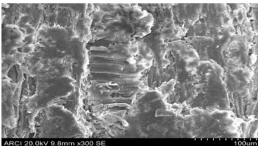
Figure 32 : Microscopic view poly acrylonitrile affinity of 4M concentration treated neem wood
