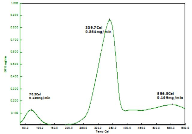
Figure 15 : D TG for Untreated cork wood
