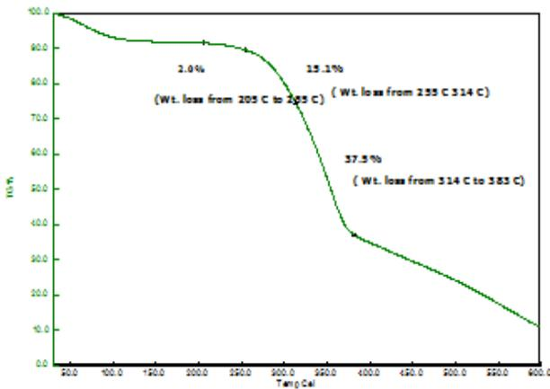
Figure 25 : TGA curve for Acrylonitrile of 6M concentrated treated cork wood
