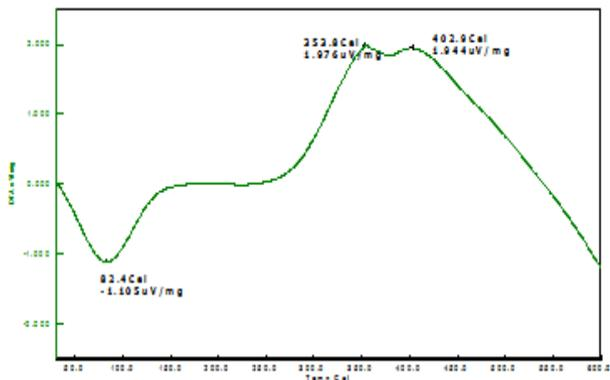
Figure 20 : DTA curve for Acrylonitrile of 4M concentrated treated cork wood
