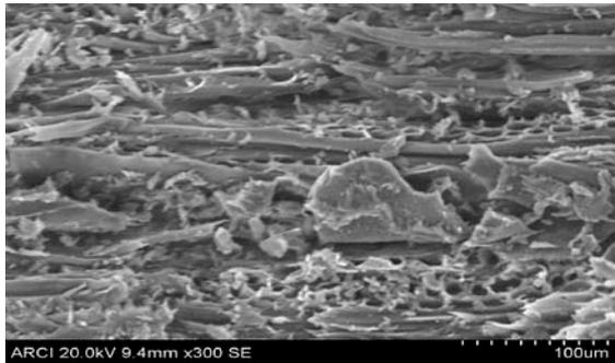
Figure 30 : Microscopic view of untreated cork wood
