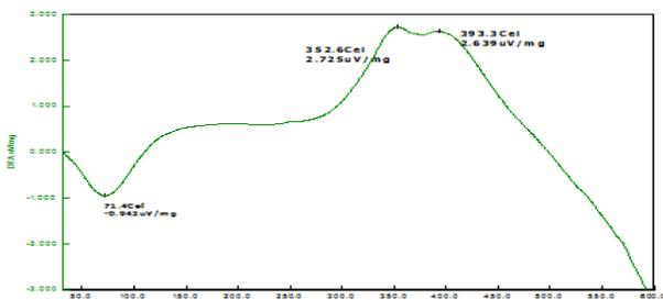
Figure 14 : DTA for Untreated cork wood
