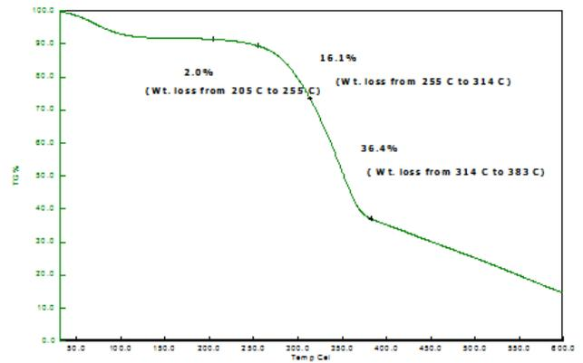
Figure 22 : TGA curve for Acrylonitrile of 4M concentrated treated cork wood
