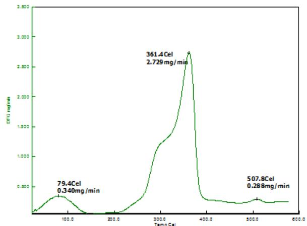
Figure 2 : D TG for Untreated neem wood
