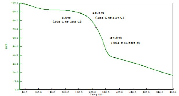
Figure 9 : TGA curve for Acrylonitrile of 4 Mconcentrated treated neem wood
