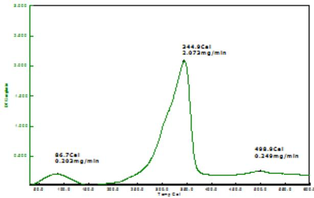
Figure 11 : DTG curve for Acrylonitrile of 6 M concentrated treated neem wood
