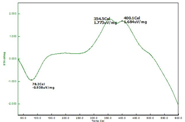
Figure 23 : DTA curve for Acrylonitrile of 6M concentrated treated cork wood
