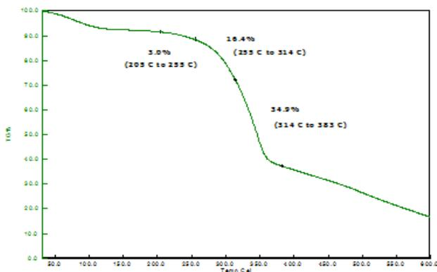
Figure 12 : TGA curve for Acrylonitrile of 6 M concentrated treated neem wood
