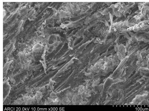
Figure 29 : Microscopic view poly acrylonitrile affinity of 6M concentration treated neem wood
