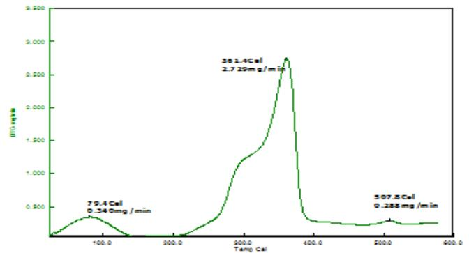
Figure 10 : DTA curve for Acrylonitrile of 4 Mconcentrated treated neem wood
