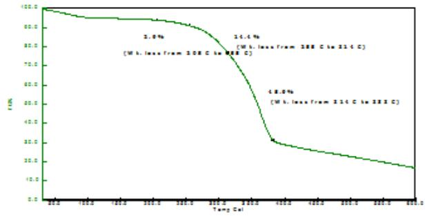
Figure 7 : TGA curve for Acrylonitrile of 2 Mconcentrated treated neem wood
