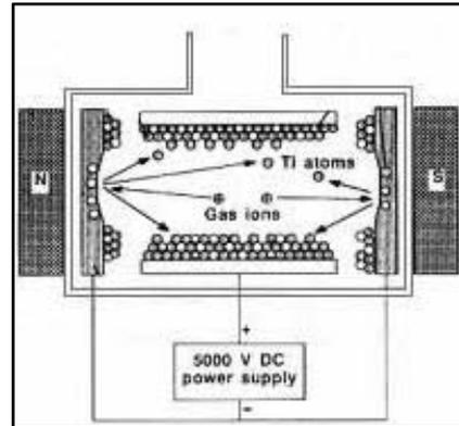
Figure 8 : Schematic of Ion Pump working principle
