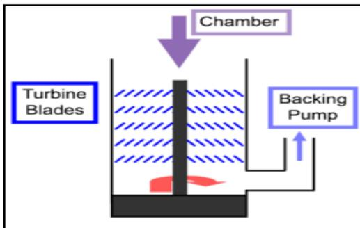
Figure 7 : Schematic of Turbo-molecular Pump working principle
