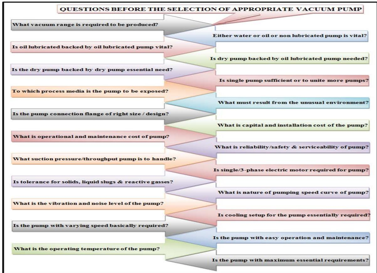
Figure 2 : Questions before the selection of proper vacuum pump
