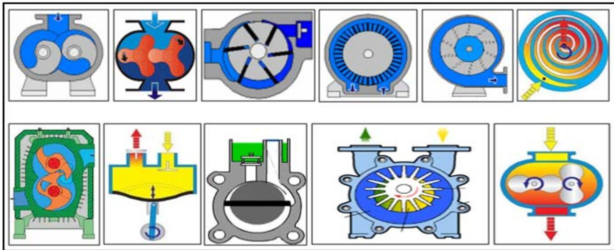
Figure 4: Schematic of working principle of some positive displacement pumps [6]
