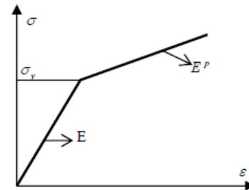
Figure 1 : Bi-linear Stress Strain Curve
