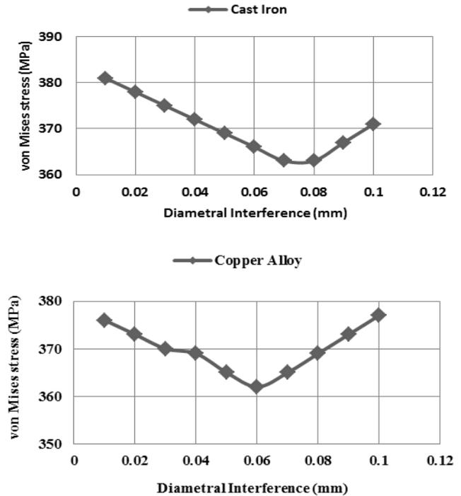
Figure 12 : Effect of different material on diametral interference (Cast iron & Copper alloy)
