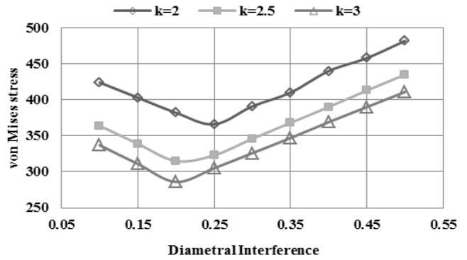
Figure 9 : Effect of k (b/a) on the diametral interference (constant inner radius = 0.1m)
