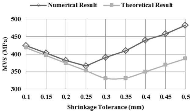
Figure 8 : Variation of MVS versus different shrinkage tolerance
