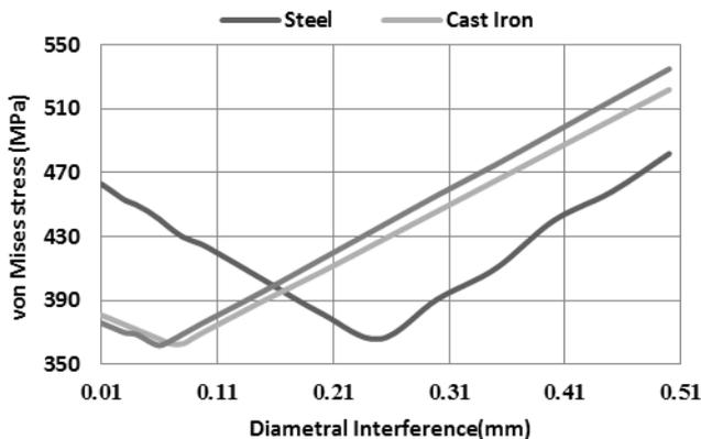
Figure 11 : Effect of different material on diametral interference
