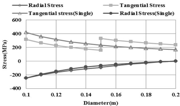
Figure 3 : Comparison of Stresses between Single & Compound Cylinder
