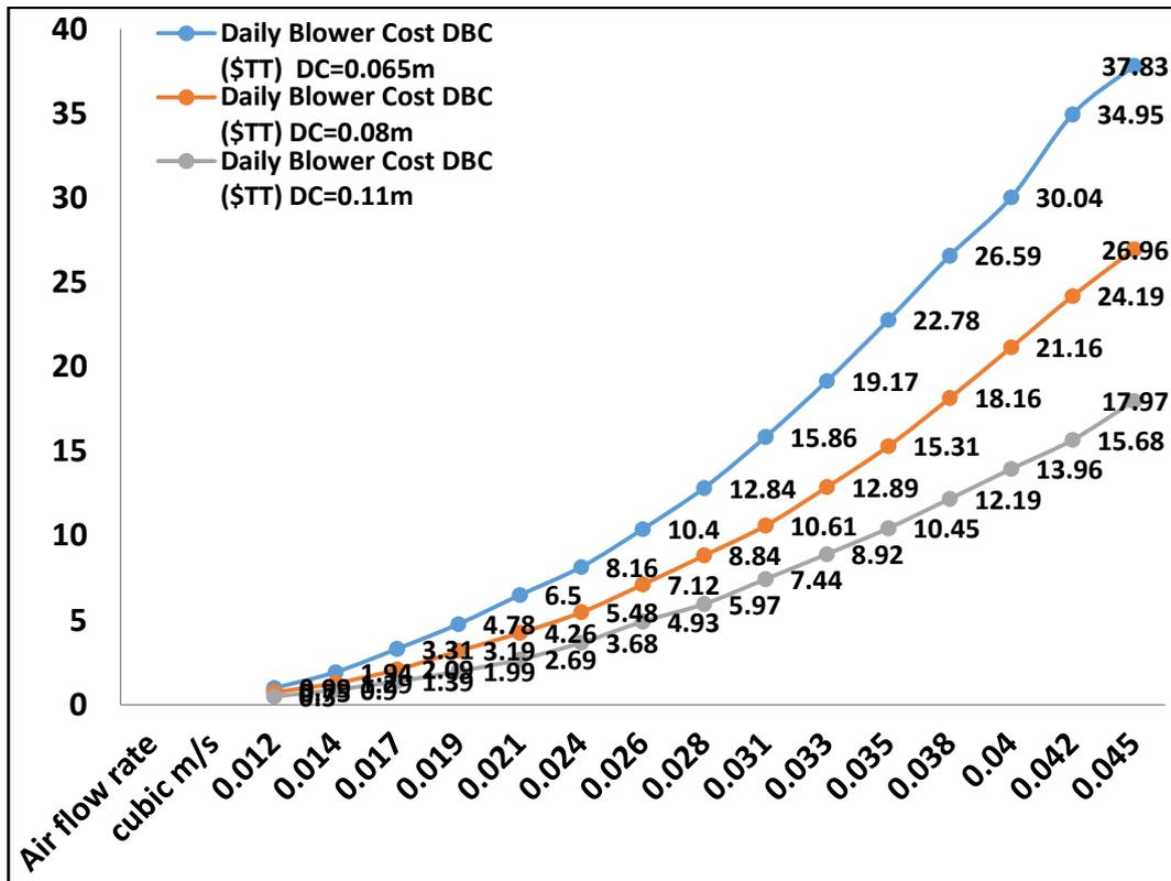
Figure 2.0 : Daily blower cost as function of air flow rate for different spherical shaped concrete of diameter 0.065, 0.08 and 0.11m
