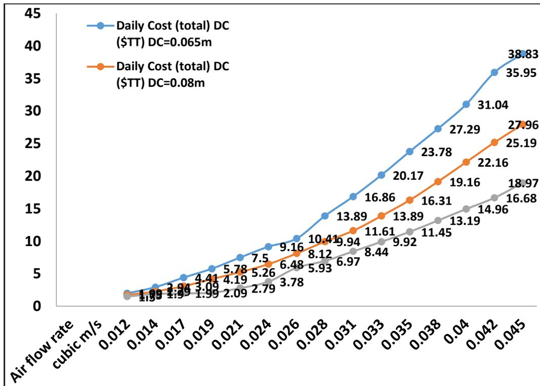
Figure 3.0 : Daily cost of the entire packed bed storage system as function of air flow rate for spherical shaped concrete of diameter 0.065, 0.08 and 0.11m
