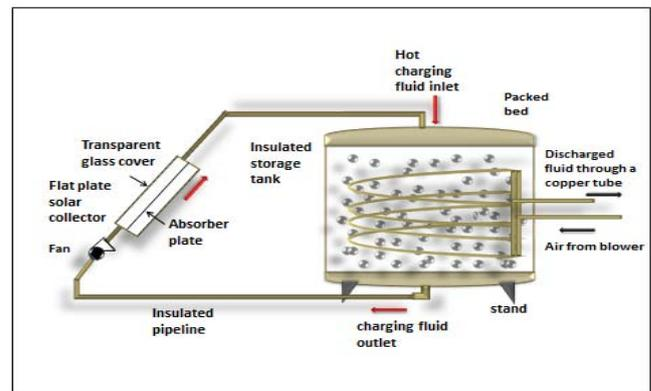
Figure 1.0 : Schematic of Combined Packed Bed Energy Storage and Solar Collector System
