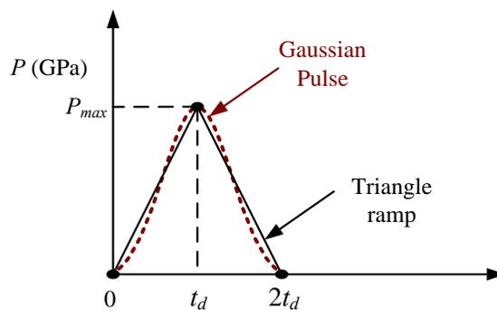
Figure 2 : Pressure-time history for LSP simulation
