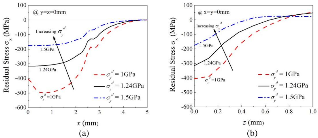
Figure 8 : Effect of the dynamic yield strength on simulated residual stress profiles
