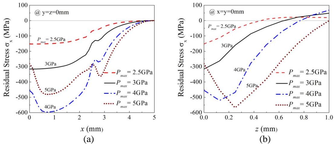
Figure 9 : Effect of the peak pressure on simulated residual stress profiles
