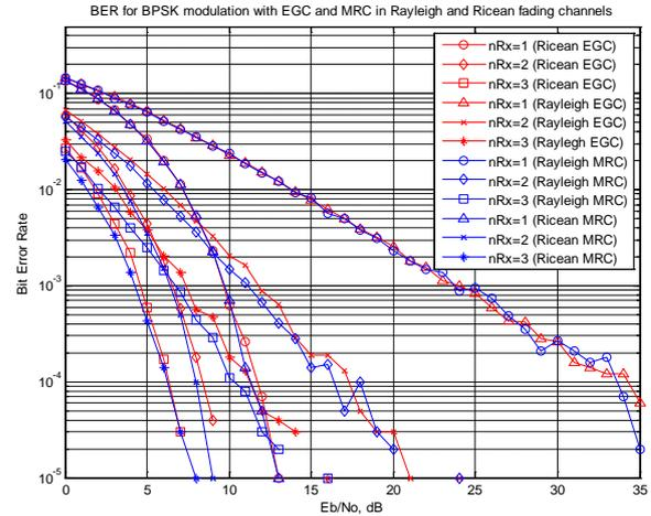
Figure 3 : BER for BPSK modulation schemes with EGC and MRC in Rayleigh and Rician fading channels
