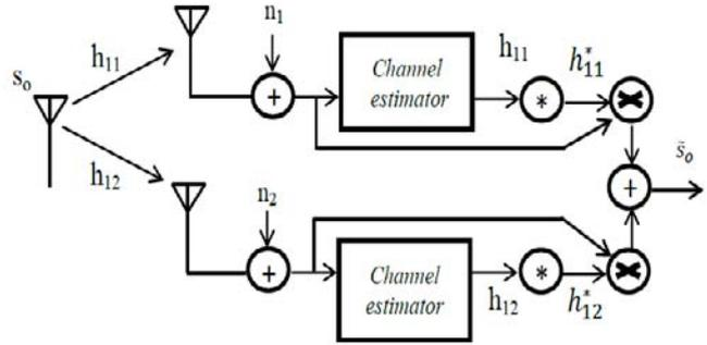
Figure 1 : MRC with 1 Tx and 2 Rx
