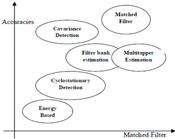
Figure 7 : Sensing accuracy and complexity of various sensing methods
