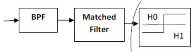
Figure 6 : Block Diagram of Matched Filter
