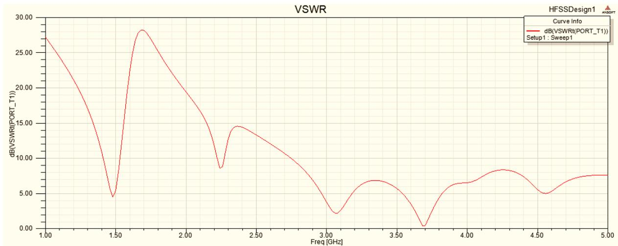
Figure 2 (b) : VSWR vs. Frequency Plot of "Antenna 1"
