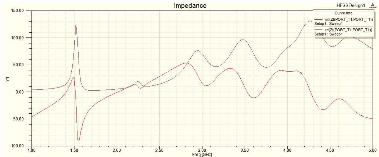
Figure 2 (c) : Impedance vs. Frequency curve of "Antenna 1"
