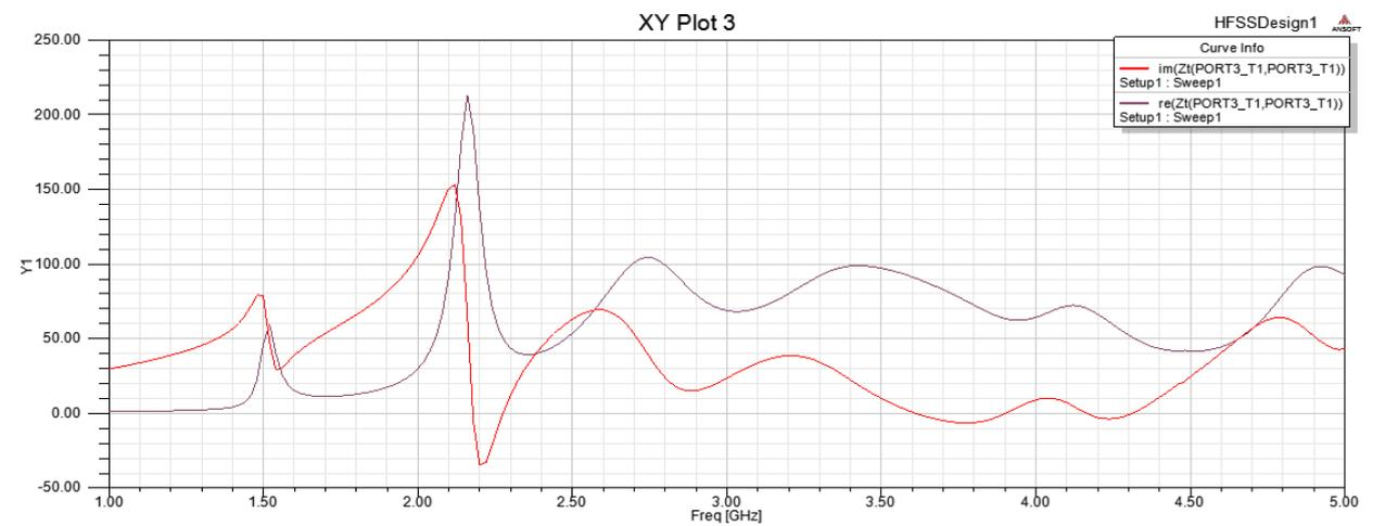
Figure 4 (c) : Impedance vs. Frequency curve of "Antenna 3"
