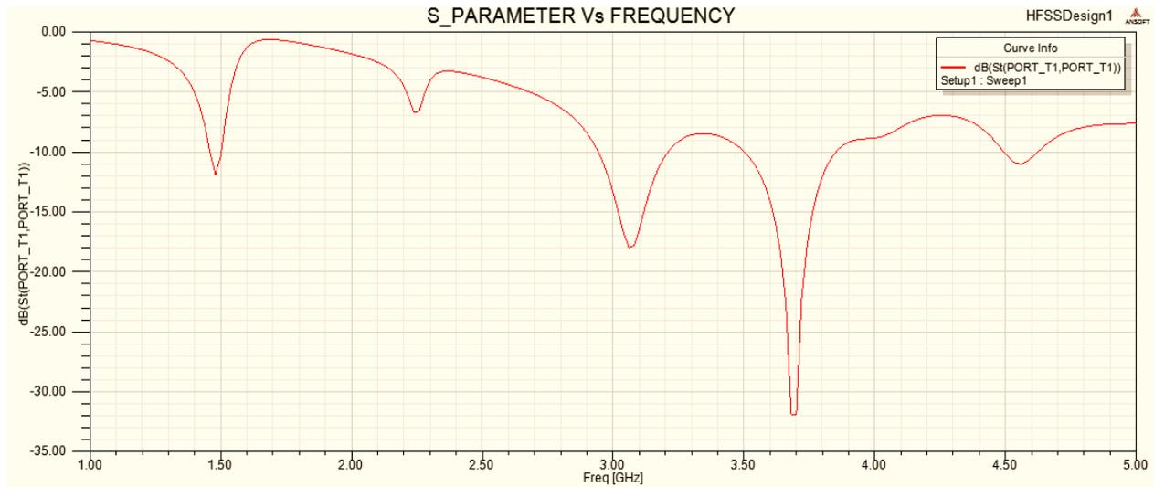
Figure 2 (a) : Return Loss Curve of "Antenna 1"
