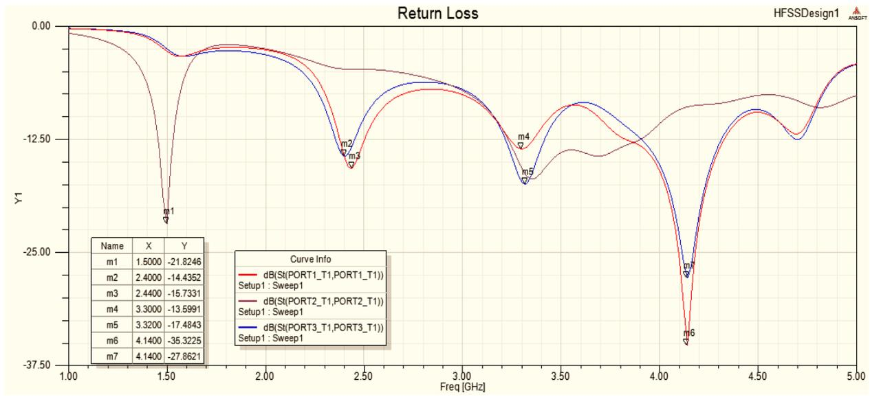
Figure 4 (a) : Return Loss Curve of "Antenna 3"
