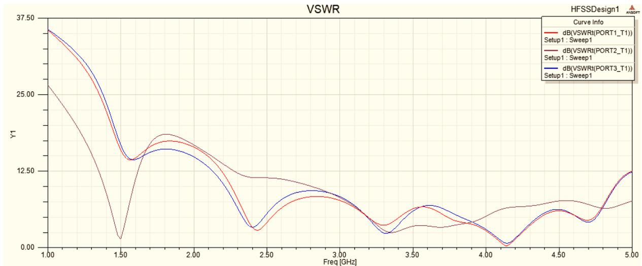
Figure 4 (b) : VSWR vs. Frequency Plot of "Antenna 3"
