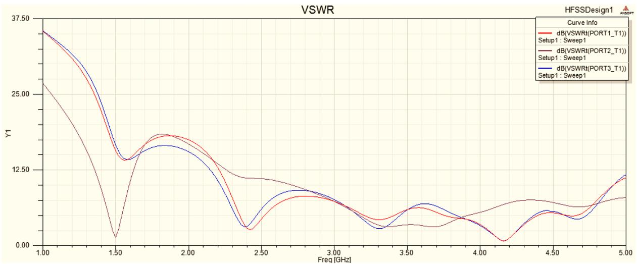
Figure 3 (b) : VSWR vs. Frequency Plot of "Antenna 2"
