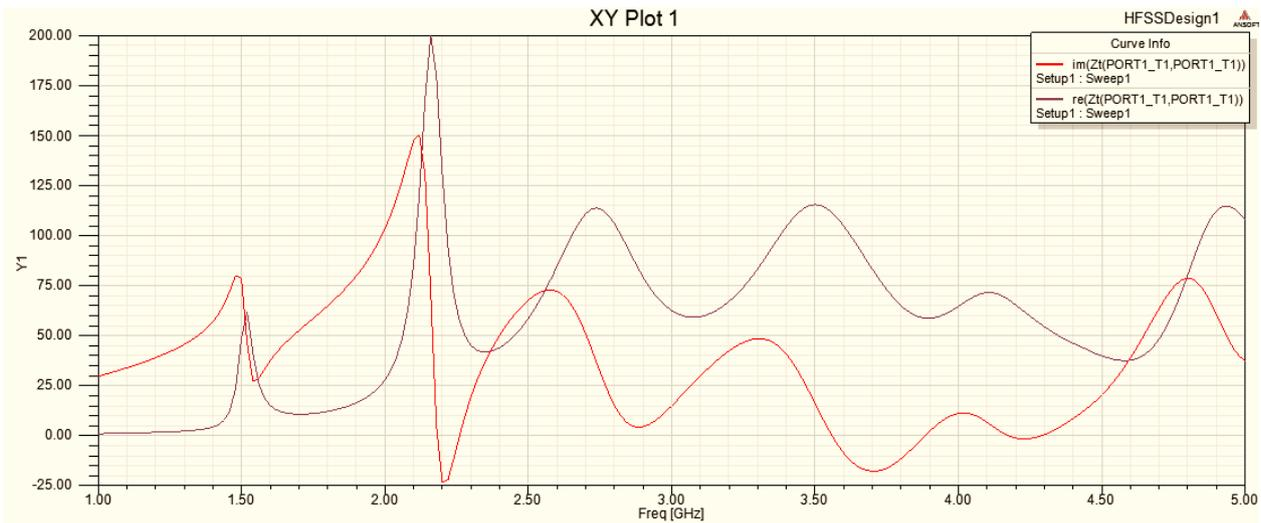
Figure 3 (c) : Impedance vs. Frequency curve of "Antenna 2"
