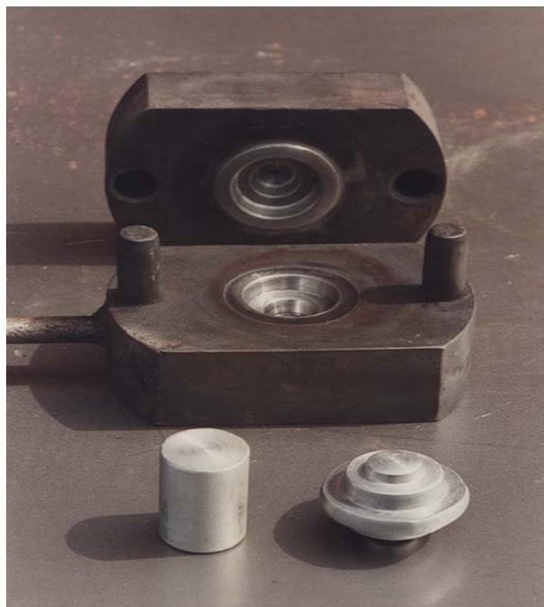
Figure 4 : Matrix, cylindrical stock material of aluminium alloy and detail forged with a rocket hammer model
