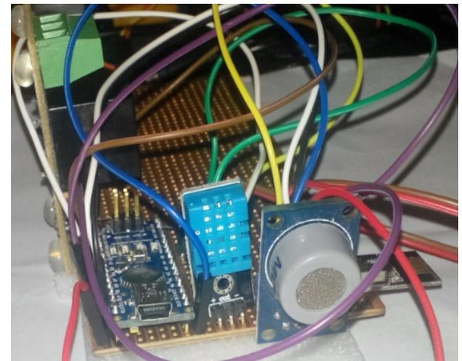
Figure 13: Sensing Node for sensing temperature and humidity
