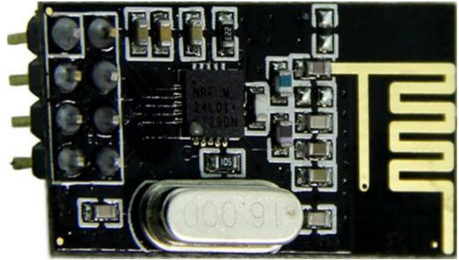
Figure 4 : NRF24L01 Transceiver
