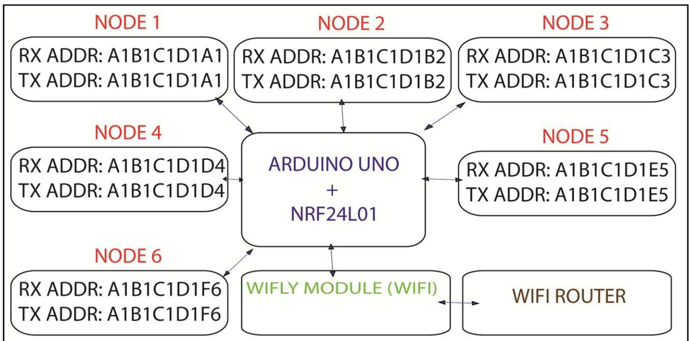
Figure 6 : Mesh networking of 6 nodes with base station
