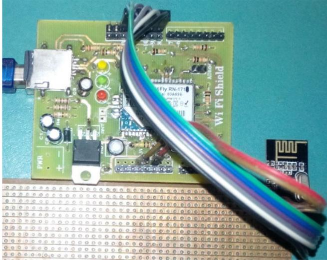
Figure 10. Hardware implementation of base station
