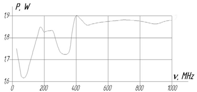
Figure 3 : Variations of power  $P$  (W) expended by friction apparatus electric motor to overcome friction forces in steady wear of friction couple “fluorine plastic-steel” in response to frequency  $\nu$  (MHz) of electromagnetic field imposed on friction unit.
