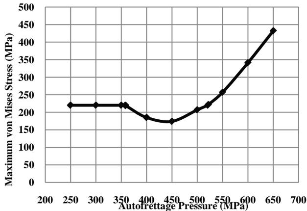
Figure 8 : Variation of Maximum von Mises Stresses at Different Autofrettage Pressure
