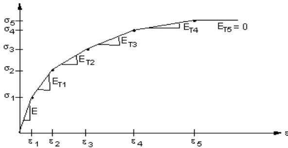
Figure 3 : Multi linear Stress Strain Curve
