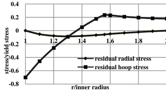
Figure 4 : Residual Stress Pattern in Autofrettaged Cylinder
