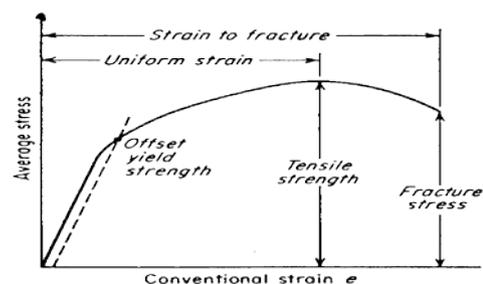
Figure 1 : Non linear Stress Strain Curve
