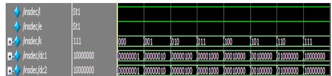
Figure 10 : Simulation Result of Instruction Decoder
