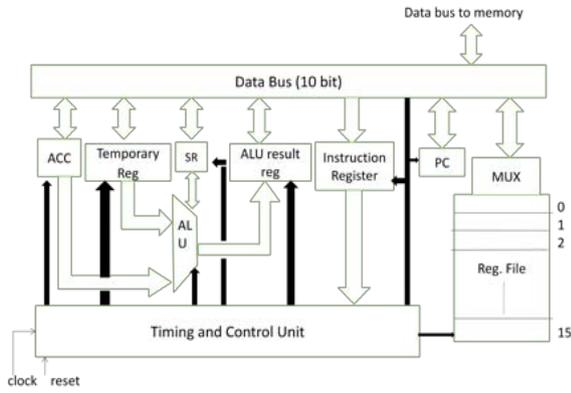
Figure 5 : Processor Architecture
