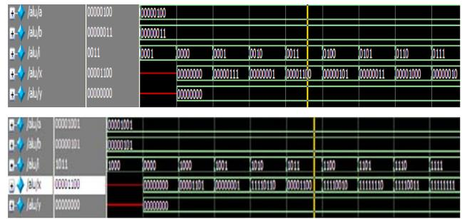
Figure 9 : Simulation Result of ALU
