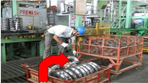
*Figure :* Excessive Bending on crown Wheel
