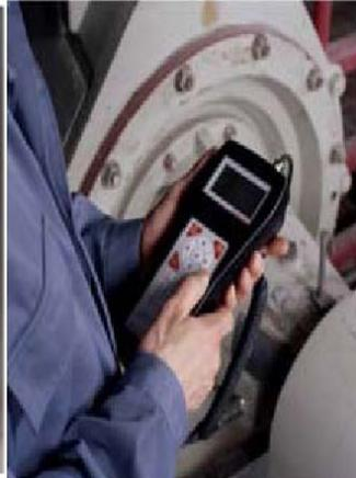
Figure 1.4 : Handheld data collector system
