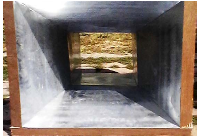
Figure 16 : Actual Contraction Cone (cross-sectional view)
