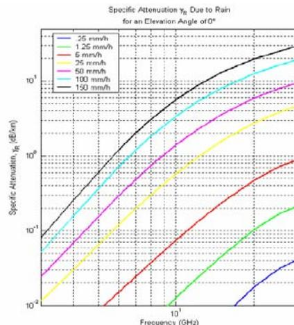
Figure 5: Specific attenuation due to rain for an elevation angle of 0°
