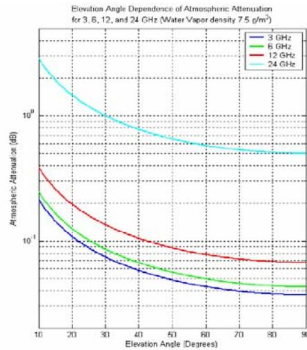
Figure 4: Elevation angle dependence of atmospheric attenuation for 3,6,12 & 24GHz (water vapor density 7.5 g/m<sup>3</sup>)
