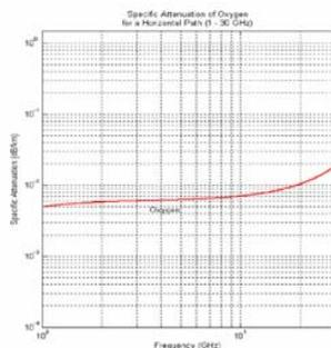
Figure 2: Specific attenuation of oxygen for a horizontal path (1-30GHz)
