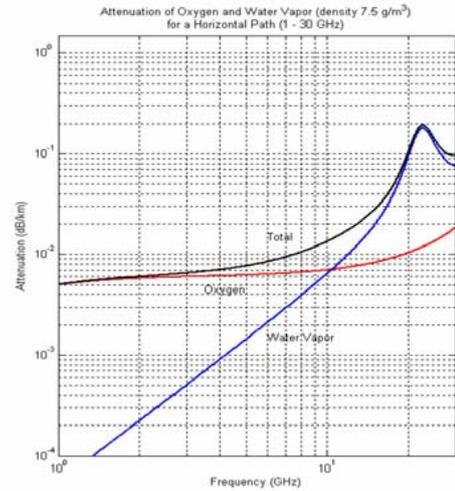
Figure 3: Attenuation of oxygen and water vapor (density 7.5 g/m<sup>3</sup>) for horizontal path (1-30GHz)
