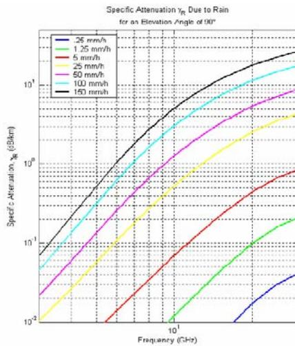
Figure 6 : Specific attenuation due to rain for an elevation angle of  $90^\circ$
