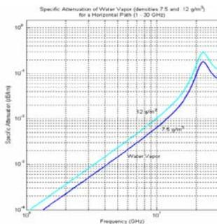
Figure 1: Specific attenuation of water vapor (densities 7.5 and 12 g/m<sup>3</sup>) for horizontal path (1-30GHz)
