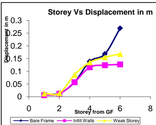
Figure 2: Story Level Vs Displacement Curve
