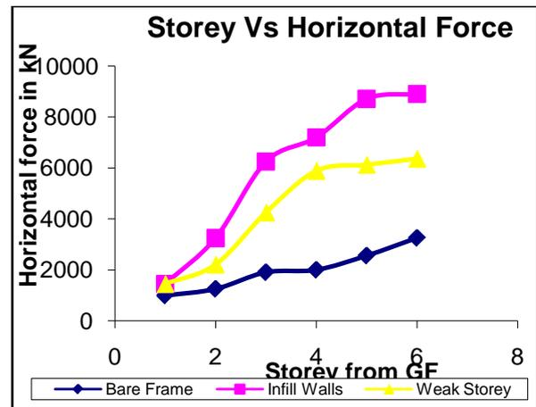
Figure 3: Story level Vs Horizontal Force Curve
