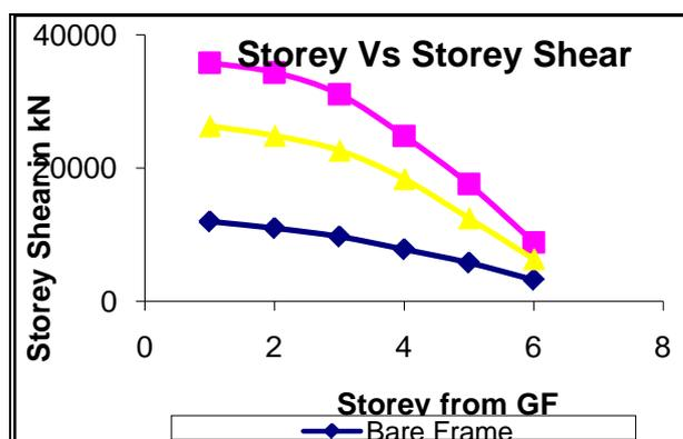
Figure 5 : Story Level from Ground Floor Vs Story Shear
