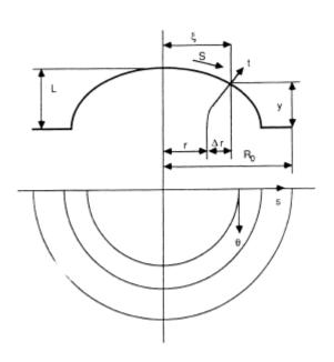
Figure 4 : Coordinates and displacement in axisymmetric sheet forming process
