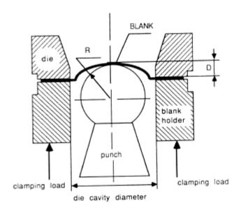
Figure 3 : Schematic illustration of Erichsen Test
