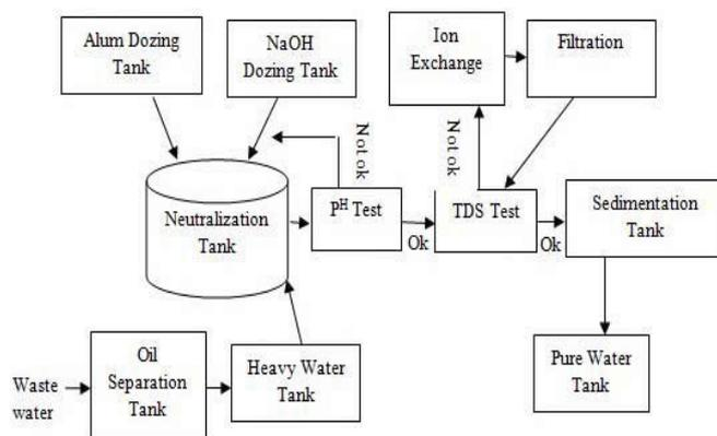
Figure 1 : Schematic block diagram of ETP
