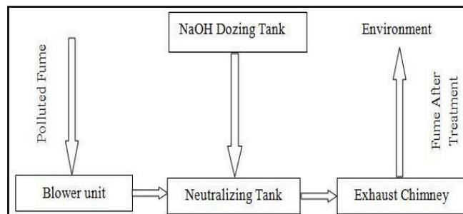
Figure 3 : Block Diagram of Fume Neutralizer Plant
