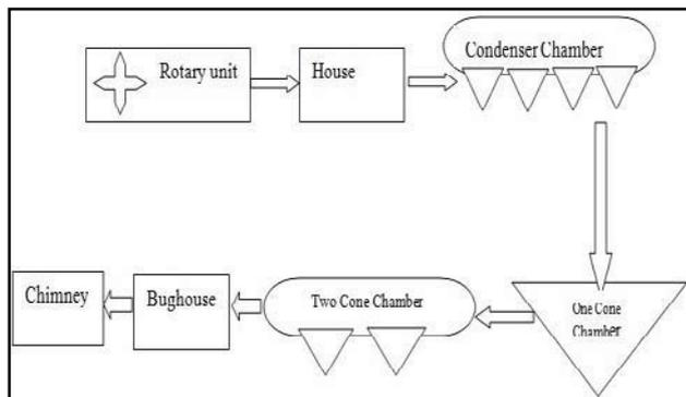
Figure 2 : Schematic block diagram of ATP
