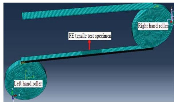
Figure 3 : Meshed model of rollers, guide plate and wire
