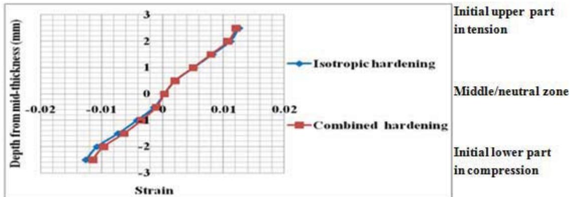
(c) Through-thickness longitudinal axial plastic strain profile
