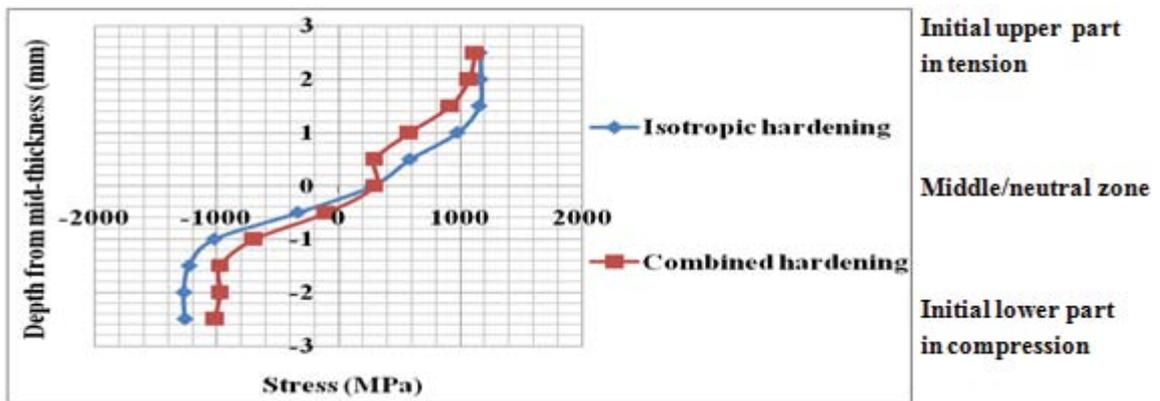
(b) Through thickness longitudinal axial stress profile
