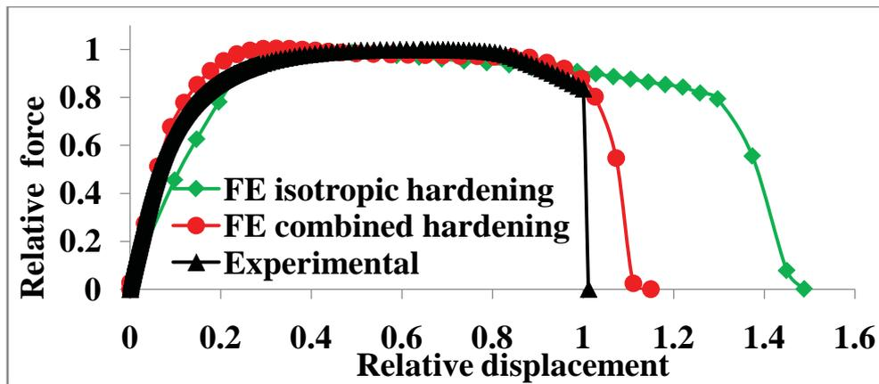
Figure 10 : Experimental and FE force-displacement curves for RBS wire specimens with isotropic and combined hardening models
