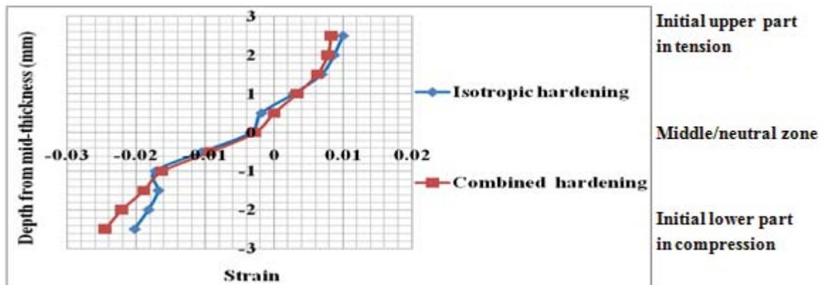
(c) Through-thickness axial plastic strain profile
