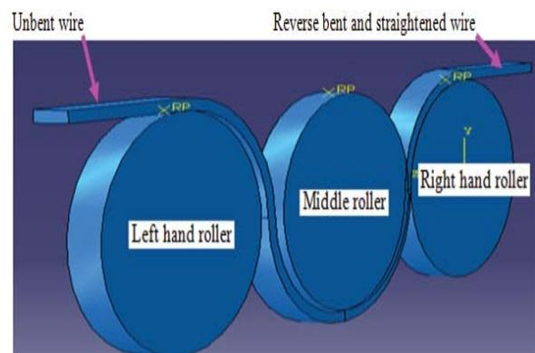
Figure 1 : Industrial reverse bending equipment with three rollers
