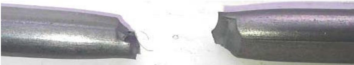
(c) Fractured experimentally RBS specimen
