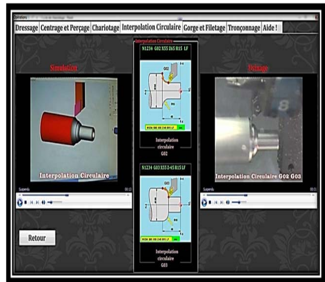
Figure 5 : Example of circular interpolation in turning
