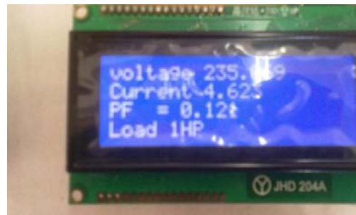
Fig. 23 : Load monitoring for 1hp inductive load
