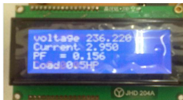
Fig. 17 : Load monitoring for 0.5hp inductive load
