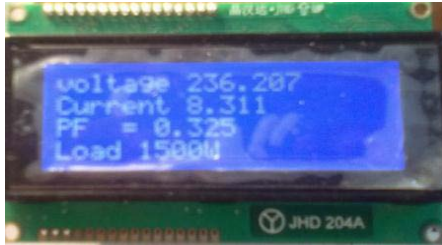
Fig. 33 : Load monitoring for resistive and inductive load
