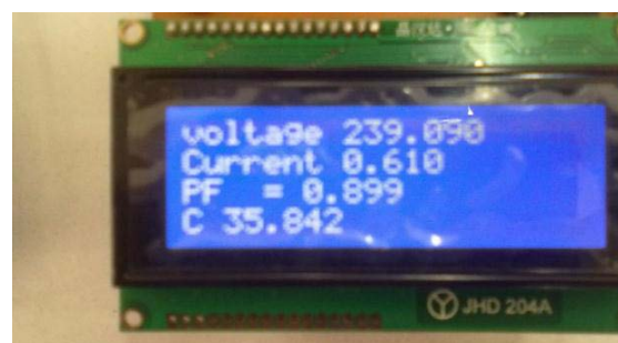
Fig. 18 : LCD showing value of 'C'
