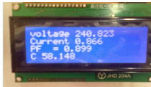
Fig. 24 : LCD showing value of 'C'
