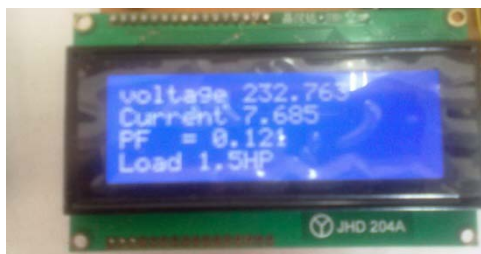
Fig. 28 : Load monitoring for 1.5hp inductive load
