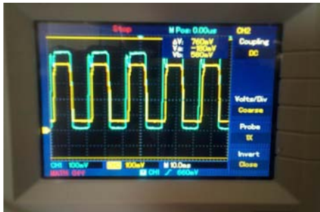
Fig. 20 : Zero crossing detection after correction with 0.5hp inductive load
