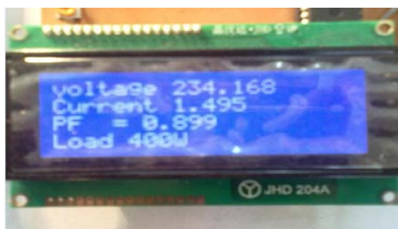
Fig. 14 : Load monitoring for resistive load
