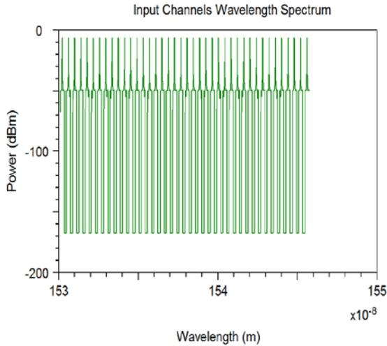
Figure 7.7 : Input channel wavelength spectrum of the 40-channel DWDM link
