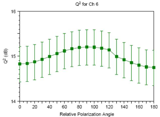
Figure 7.2 (b) : Channel performance versus polarization angle between adjacent channels: Even channel example (ch.6)
