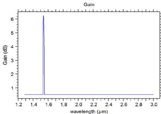
Figure 7.4 : Frequency response of the 40-channel DWDM link
