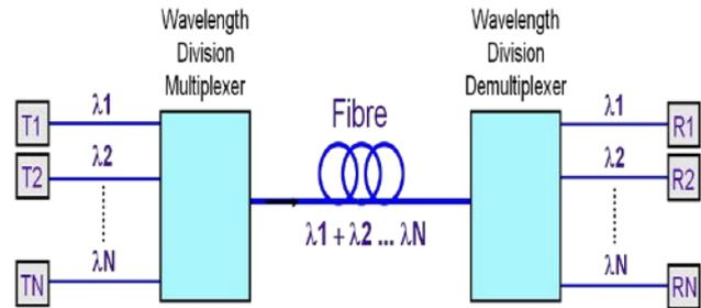
Figure 3.1 : Simple block diagram of DWDM system having N-inputs and N-outputs
