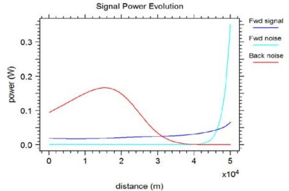
Figure 7.9 : Signal power and noise power over the distance of the fiber in the 40-channel DWDM link
