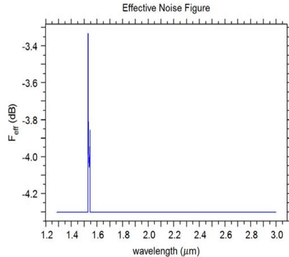
Figure 7.6 : Noise figure versus wavelength plot of the 40-channel DWDM link
