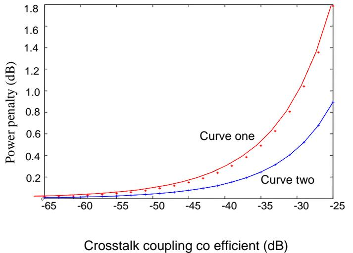
Figure 7.1 : Relation between power penalty and crosstalk coupling coefficient
