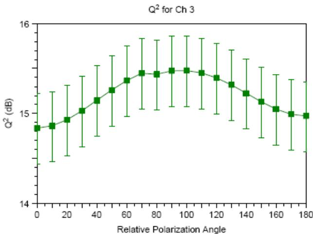
Figure 7.2 (a) : Channel performance versus polarization angle between adjacent channels: Odd channel example (ch.3)
