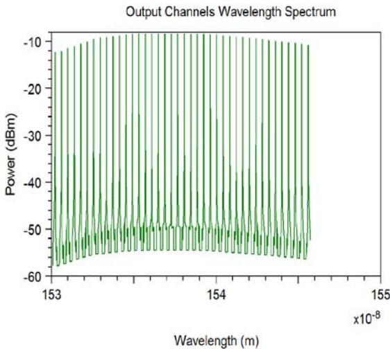
Figure 7.8 : Output channel wavelength spectrum of the 40-channel DWDM link
