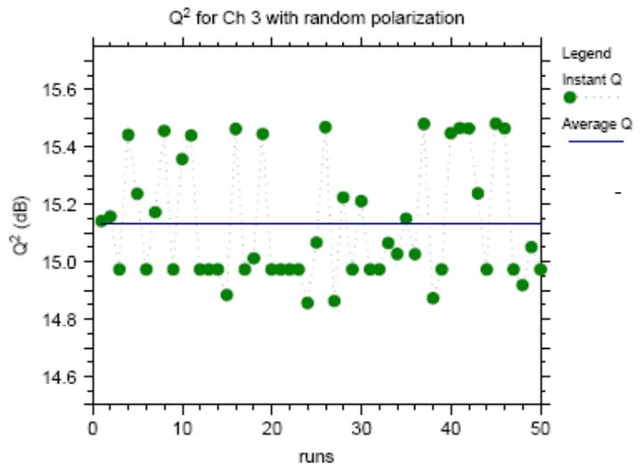
Figure 7.3 (a) : Channel performance statistics for randomly changing polarization angle between adjacent channels: Odd channel example (ch.3)
