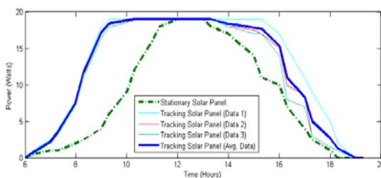
Fig. 7 : Power producing versus time of stationary solar panel and tracking panel.
