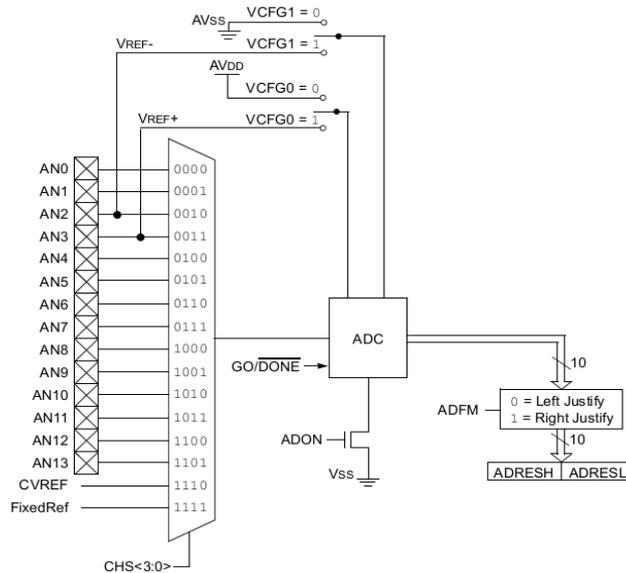
Fig. 3 : Shows the block diagram of the ADC of PIC16F72 [15].
