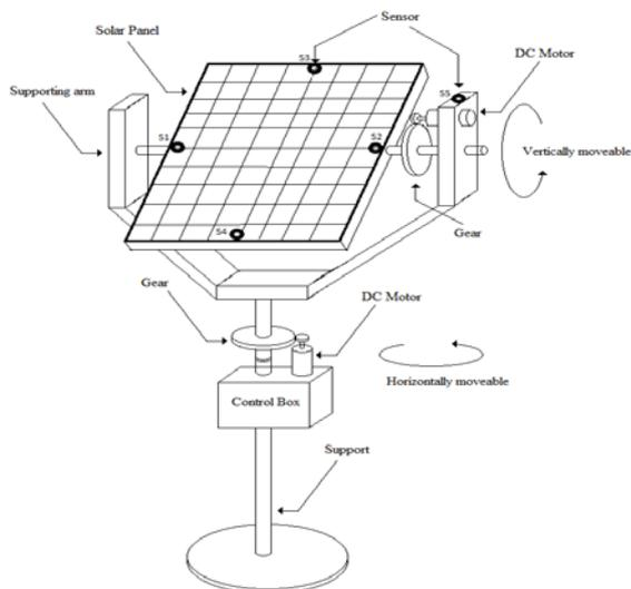
Fig. 1 : Structural view of two ways rotating freedom solar tracker.
