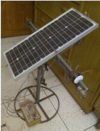
Fig. 6 : Practical view solar Tracker by Using ADC of Microcontroller
