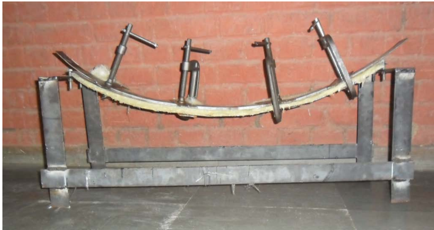
Fig. 5.1 : E-glass/ Epoxy composite leaf spring curing on the mould set up.
